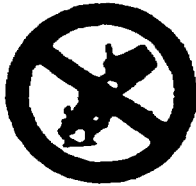
Do not extinguish with water
