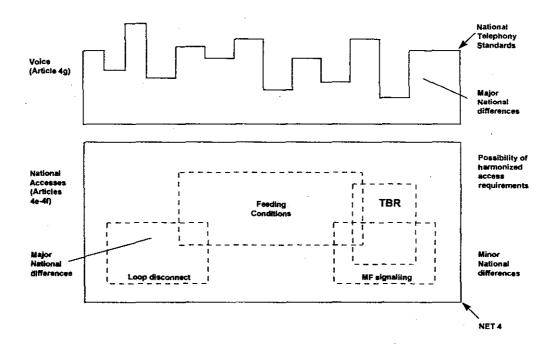
The diagram shows how a TBR for terminal with features such as low drain and MF signalling can find a possibility of harmonised access requirements by avoiding areas where there are major national differences. This approach means harmonisation can be found within the existing requirements, without having to harmonise the content of NET 4 or of national telephone requirements.
