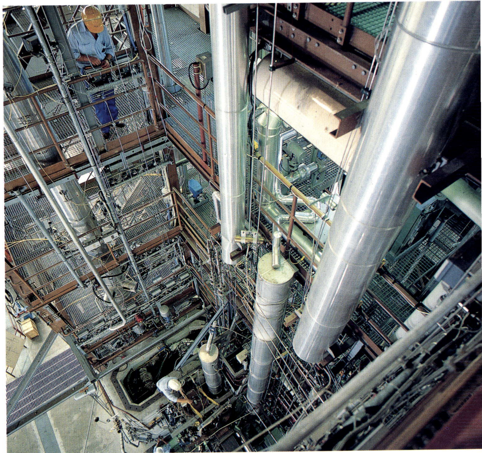
Figure 30: The LOBI experimental facility used for integral tests on loss of coolant accidents in Light Water Reactors
