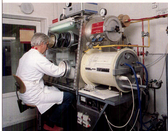
Figure 6: General view of the preparation unit for synthetic uranium isotope mixtures
