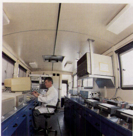
Figure 78: An interior view of the mobile unit used for in-field analysis of atmospheric pollutants
