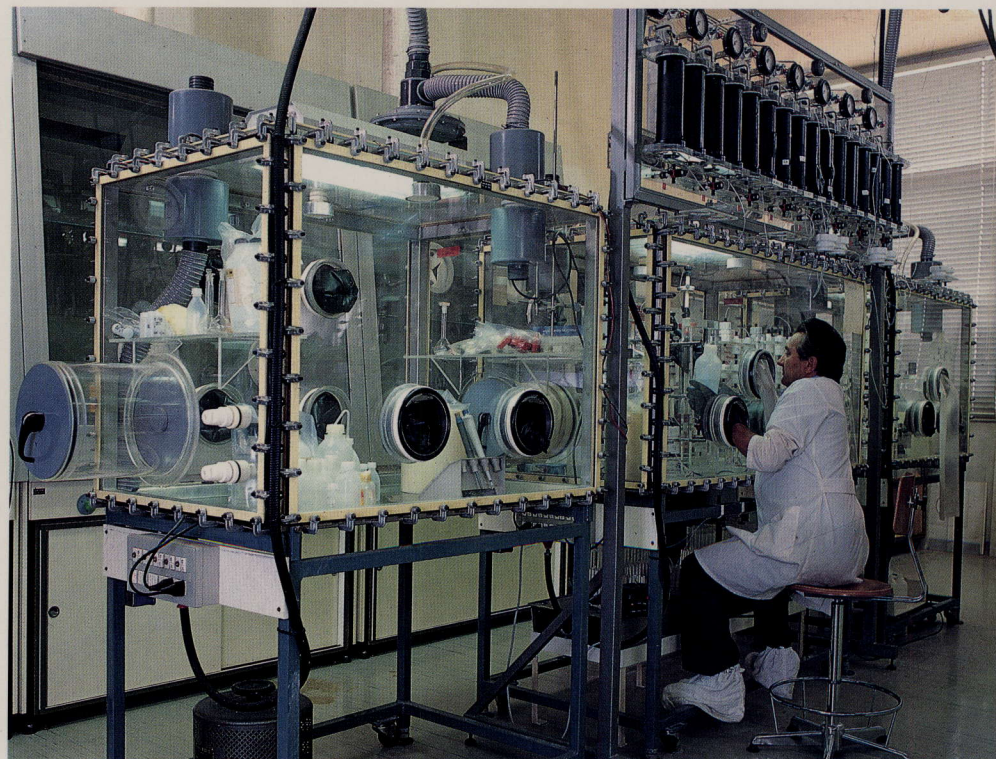
Figure 44: Laboratory simulation experiments on geochemical migration of radionuclides using groundwaters and geological materials typical of the different disposal options considered
