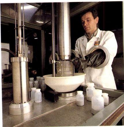
Figure 36: Examination of the particle distribution on a debris bed carried out as part of the PAHR in-pile tests
