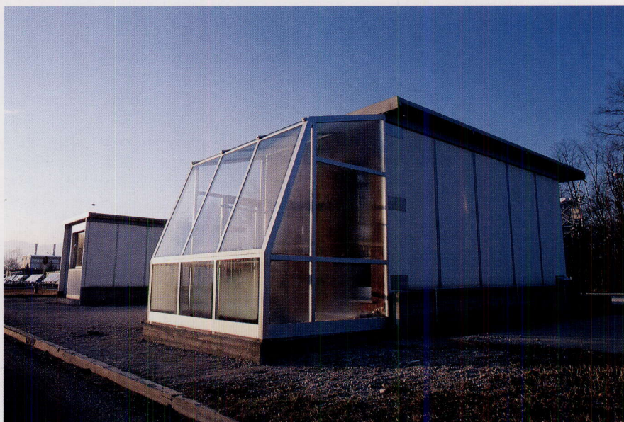
Figure 70: One of a group of passive solar test cells which make up the extensive test facility installed at the Ispra establishment
