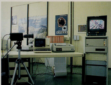
Figure 51: The computer vision system for reviewing images obtained during optical surveillance. The pictures are grabbed by the TV camera, processed by the computer and displayed on the TV monitor
