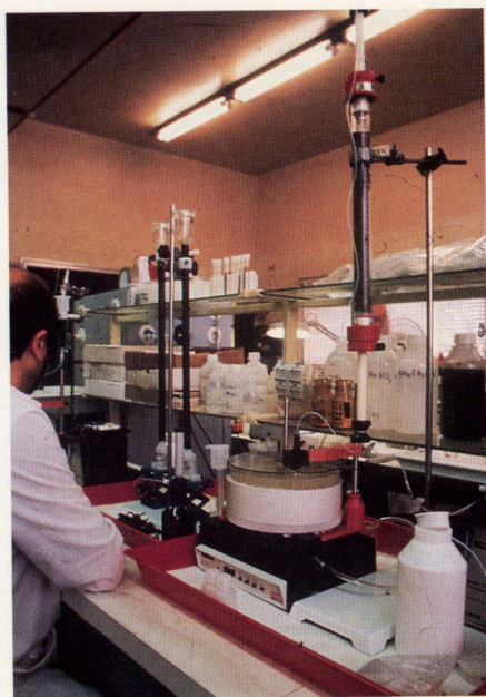
Figure 76: Environmental pathway of trace metals; laboratory leaching experiments on fly ashes by radioactive tracers
