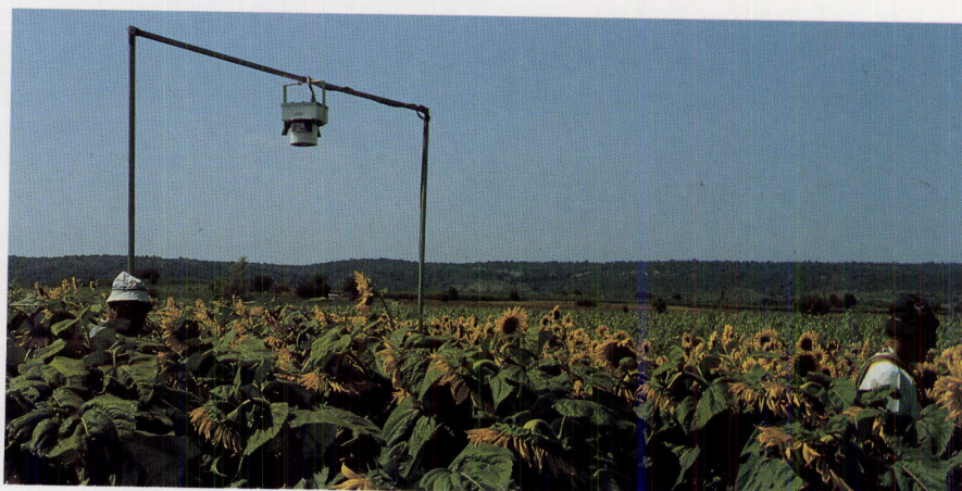
Figure 86: Radiometric measurements made over a sunflower crop by means of a radiometer with the same spectral bands as the Thematic Mapper Satellite
