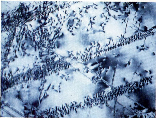
Figure 13: A bright field TEM image of planar array of partial dislocations after 10% deformation at 373 K
