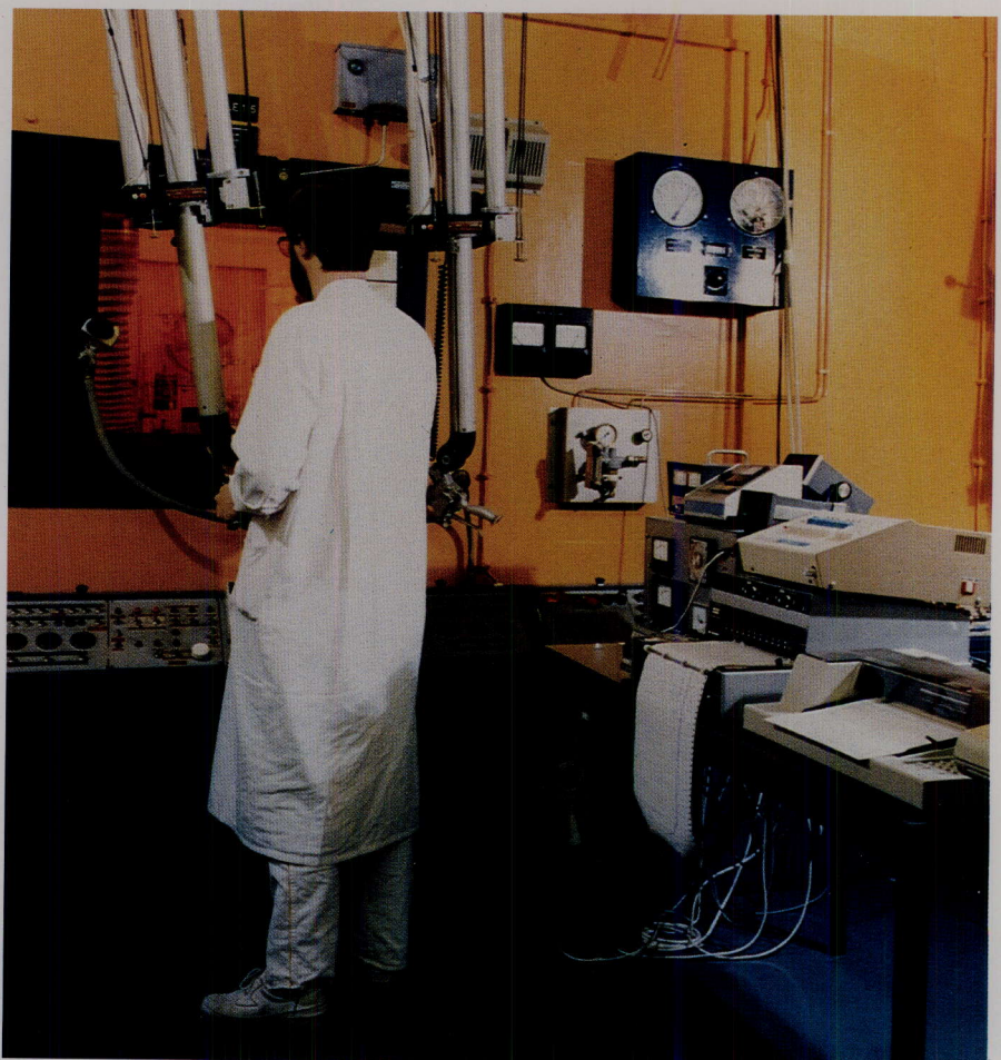
Figure 58: A view of an \alpha, \beta, \gamma cell of the hot cell facilities used for non destructive analysis in the dissolution of spent fuel samples
