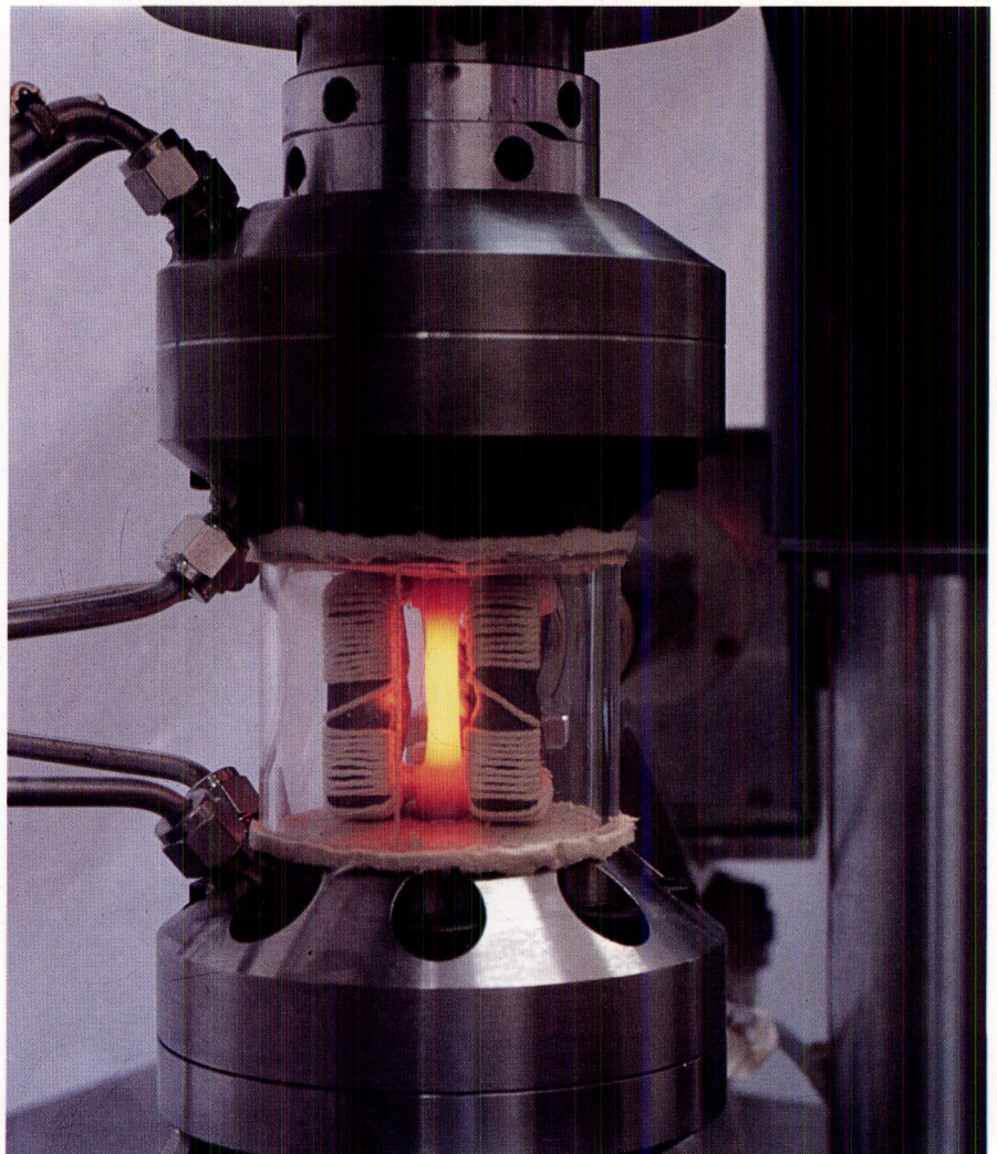
Figure 9: View of an induction heated specimen in a low cycle fatigue test rig
