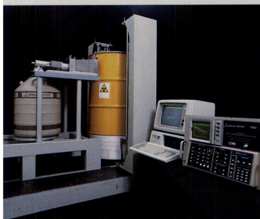
Figure 43: High sensitivity segmented \gamma scanner for determination of the Pu-isotope composition of waste barrels
