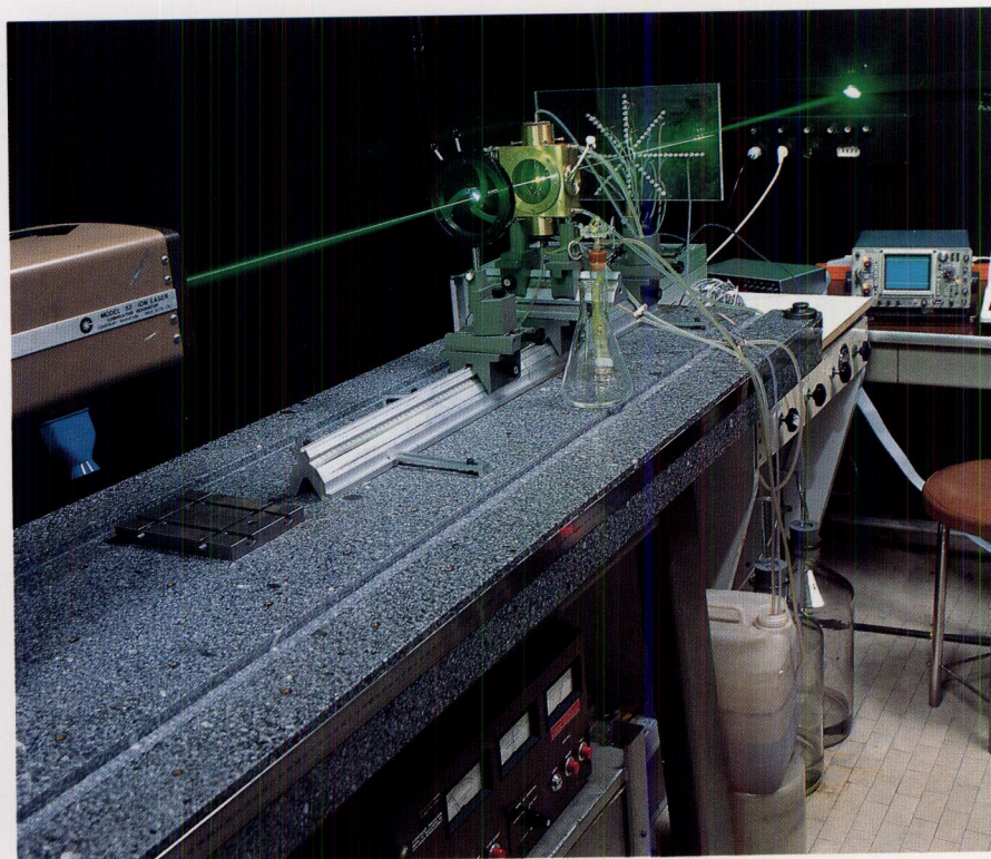
Figure 82: Laser diffraction flow cytometry for measuring the evaluation of the algal biomass in a fresh water ecosystem
