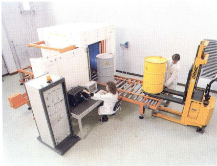
Figure 30: Neutron counting techniques have been developed to monitor the actinide content in solid waste, non destructively.
