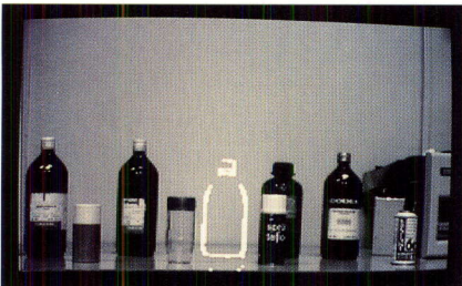
Figure 54: A computer vision system demonstrates here a scene modification (missing object is shown by white contour lines) during a surveillance of fissile materials stored in a cell.
