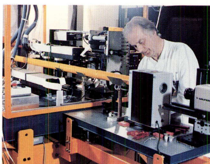
Figure 8: Laser and pyrometer for thermophysical property measurements at very high temperatures
