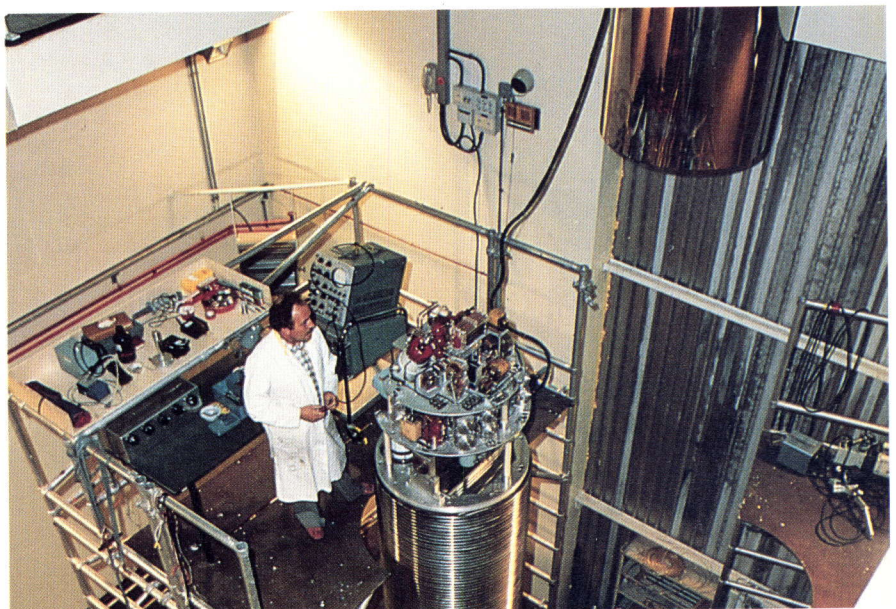
Figure 79: The 3.7 MV Van de Graaff accelerator at the CBNM used for nuclear measurements and the assay of trace elements
