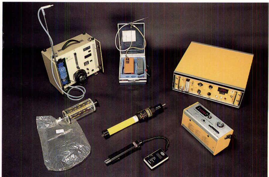
Figure 16: Portable instrumentation for field investigations of indoor air quality. From left to right - above: 1) adsorption/reaction cartridge and metering pump for the air sampling of aldehydes; 2) same for volatile organic compounds (VOC); 3) portable chromatograph for tracer gas measurements; below: 4) bag and gas syringe for tracer gas sampling; 5) photoionization detector for the measurement of total VOC; 6) temperature and humidity meter; 7) monitor for respirable particulate matter.
