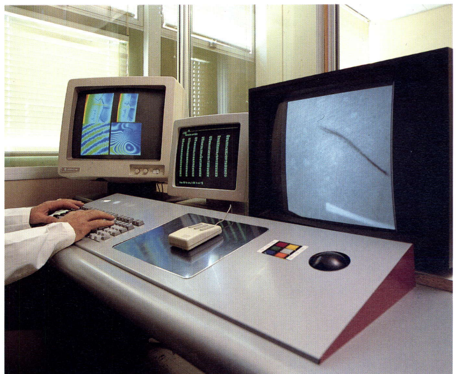
Figure 61: VICOR Image Processing: studies of crack growth by analysing high density X-ray negatives. These negatives are digitized using a high efficiency in-house negatoscope and then stored on high speed hard disks. The system has zooming capabilities up to 60 times enlargement.
