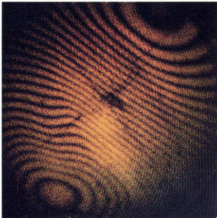
Figure 60: Laser interferogram of a pipe interior, obtained by optical fibres
