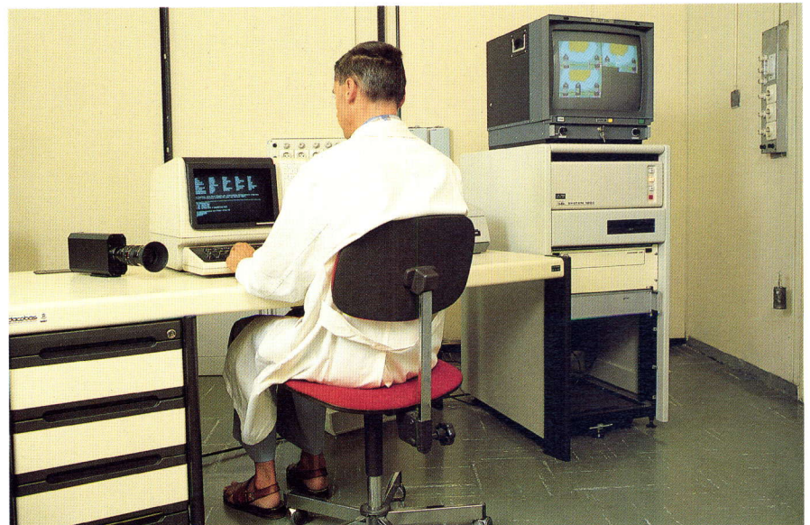
Figure 53: The computer vision system for reviewing images obtained during optical surveillance. The pictures are grabbed by the TV camera, processed by the computer and displayed on the TV monitor.
