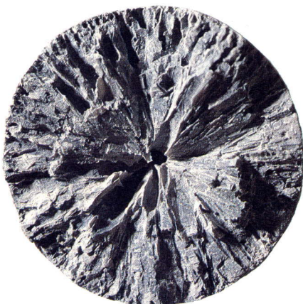
Figure 51: Breeding material ( \text{Li}_{17}\text{Pb} ) after simulation of a steam generator accident in a fusion reactor liquid metal blanket
