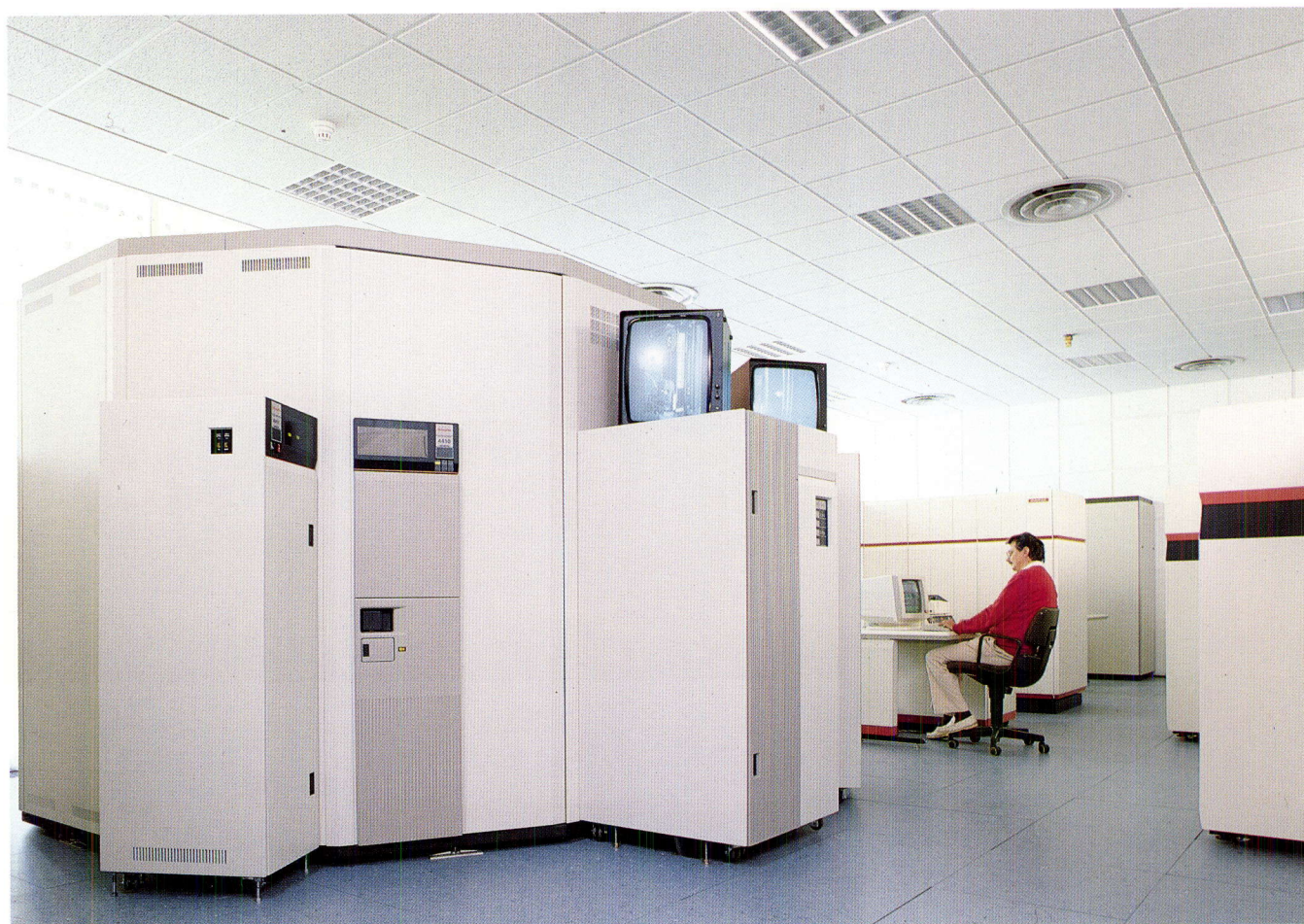
Figure 85: Automated tape cartridge library containing 1200 Gigabytes of archival data with robot-controlled access plus 'juke box' optical disk archive (worm) with 300 Gigabytes of data
