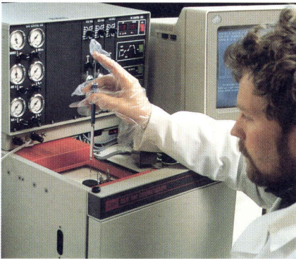
Figure 72: Analysis of toxic PCBs in oil by dual-column high resolution gas chromatography
