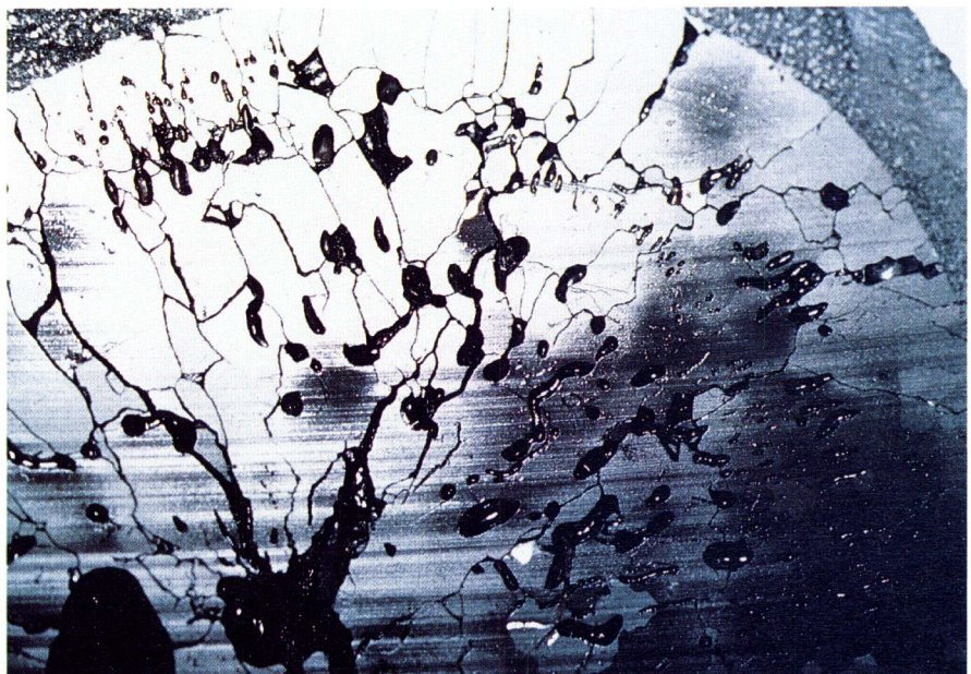
Figure 41: Microgram from a part of a solidified UO 2 block after melting in the FARO furnace.
