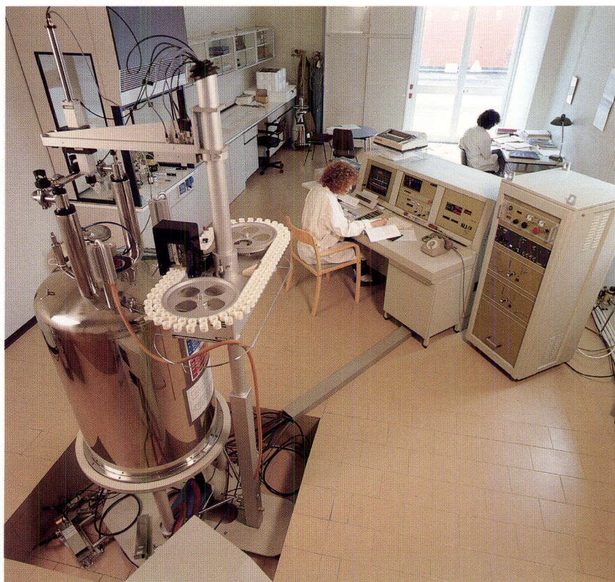
Figure 68: The new 300 MHz Nuclear Magnetic Resonance Spectrometer. Measurements taken of the deuterium/hydrogen ratio in the different sites of ethanol, derived from wine or other alcoholic beverages, permit the determination of its history and origin.
