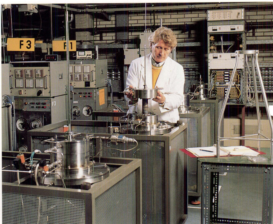
Figure 11: Autoclaves for high temperature corrosion studies
