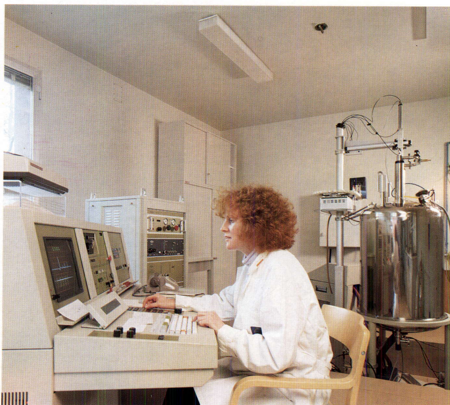
Figure 34: The 300 MHz Nuclear Magnetic Resonance Spectrometer used to determine the history and origin of the alcoholic content of wines and other alcoholic beverages.
