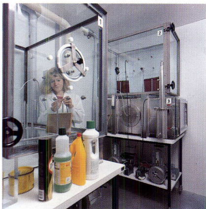
Figure 23: Thermostated room with three chambers, two made of glass and one of stainless steel, for the measurement of organic emissions from building materials, household and hobby products.
