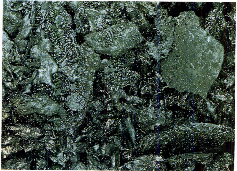
Figure 50: FARO-UO 2 collected upon release from the furnace after interaction with a stainless steel plate.
