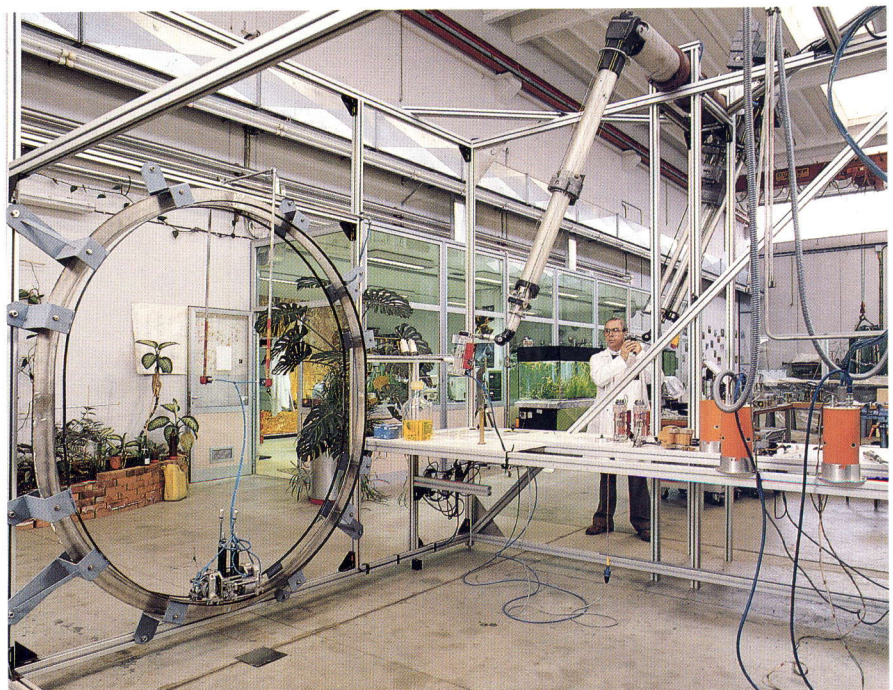
Figure 17: A view of the Remote Handling Laboratory with the Manipulator Test Bench used to simulate handling procedures of internal components in support of design studies on ITER.
