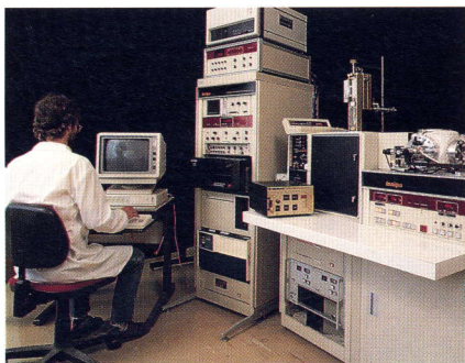
Figure 25: Laboratory configuration for the introduction of VOC samples into the gas chromatograph by way of a thermal desorption cold trap injector.
