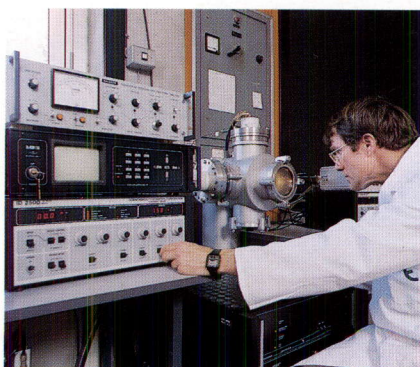
Figure 9: A dual ion beam sputter device used in surface materials studies.
