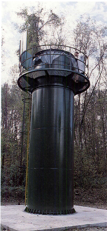
Figure 44: A 7 metre high tank used to simulate LIDAR measurements on a water column.
