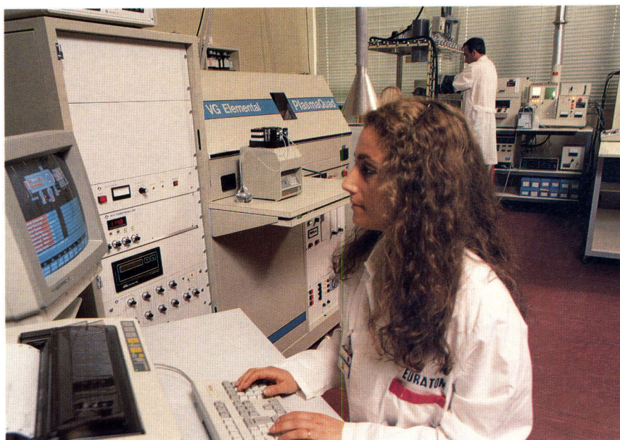
Figure 36: A view of the laboratory housing the Inductively Coupled Plasma Mass Spectrometer (ICP-MS) used in chemical waste research activities.
