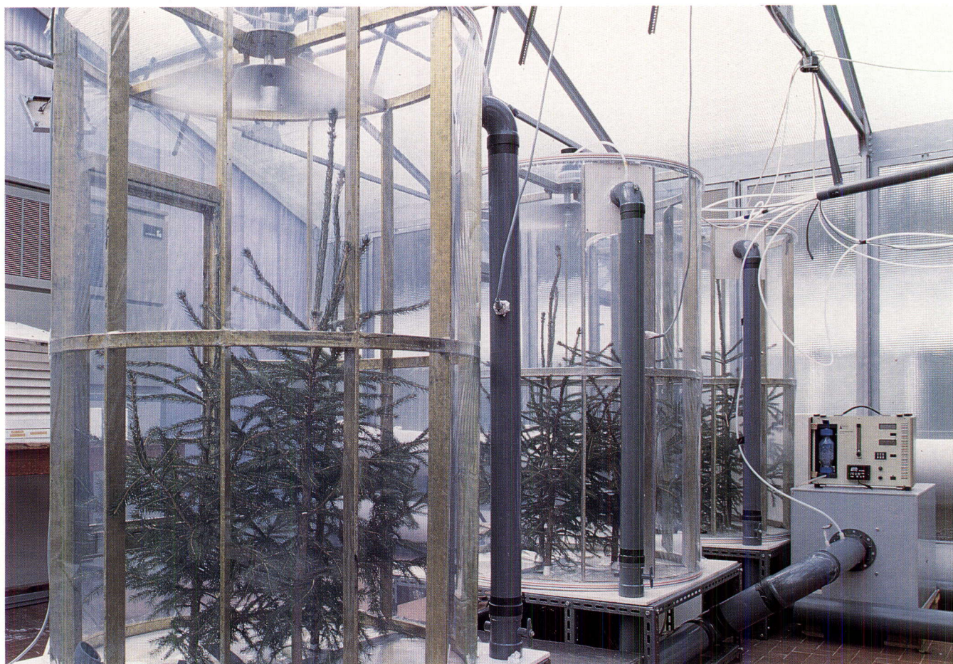
Figure 27: Deposition studies: continuous stirred tank reactor for fumigation of plants with mixtures of atmospheric pollutants.
