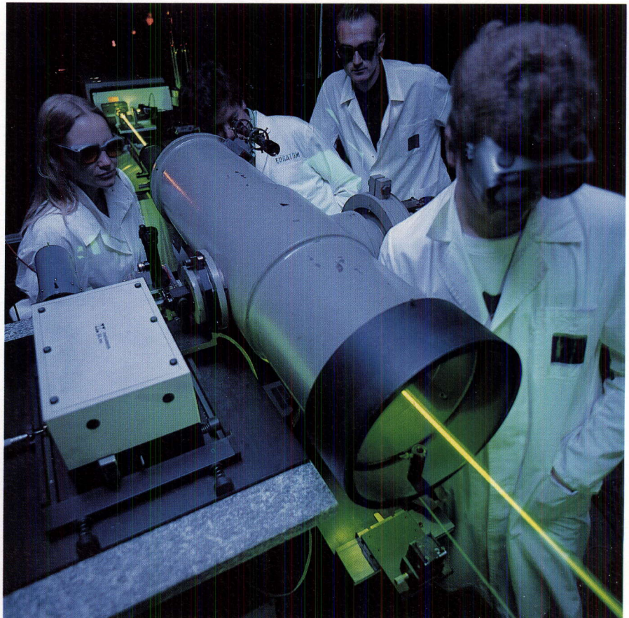
Figure 43: The excitation laser and receiving telescope used for fluorescence light collection which forms a part of the LIDAR Fluorosensor Facility's analysis of remote targets in environmental investigations.
