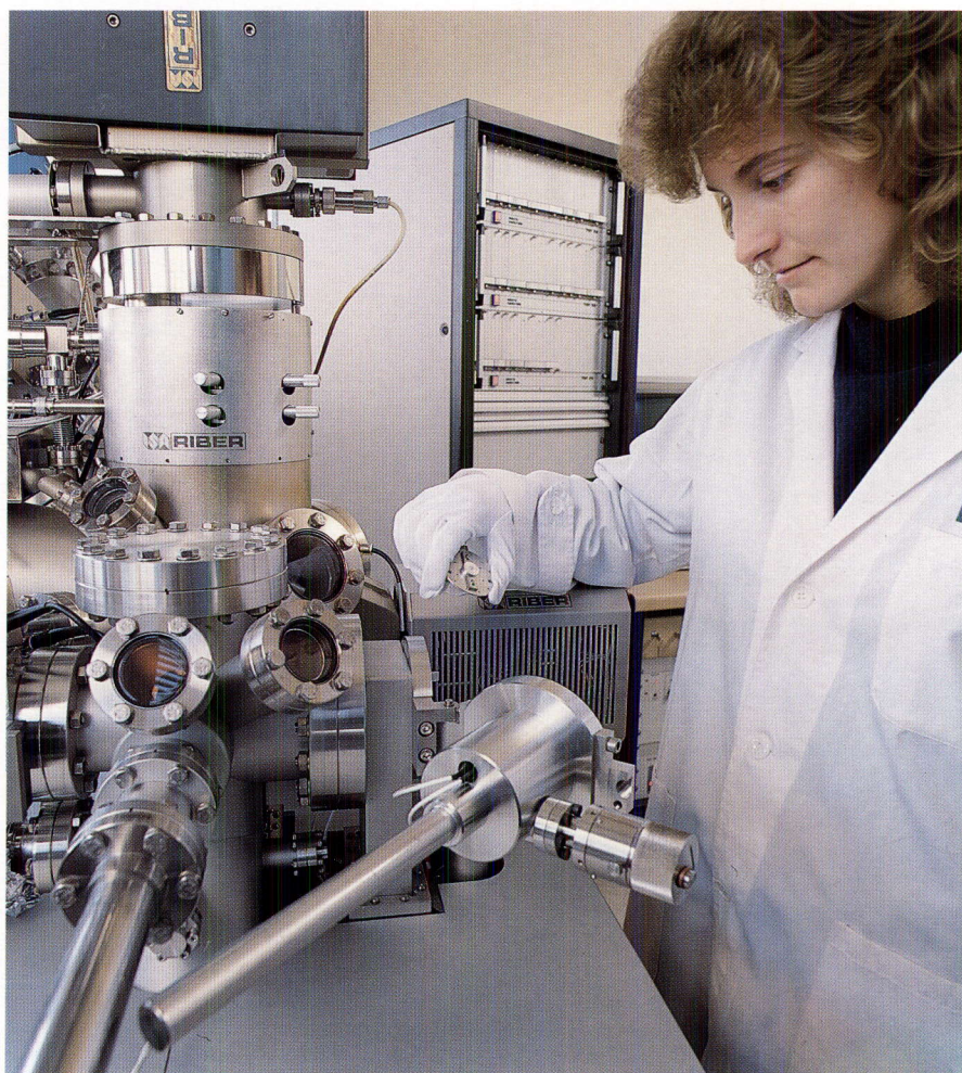
Figure 8: Mounting a sample into the SAM (Scanning Auger Microscope) preparation chamber for surface materials studies.
