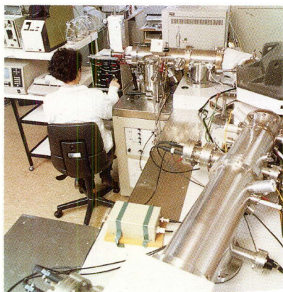
On-line capillary high pressure liquid chromatograph - Fandem Mass Spectrometry for the detection of trace and ultra-trace amounts in environmental and food and drug analysis
