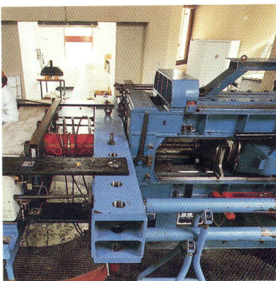
The Large Dynamic Test Facility (LDTF) in preparation for testing reinforced concrete beams
