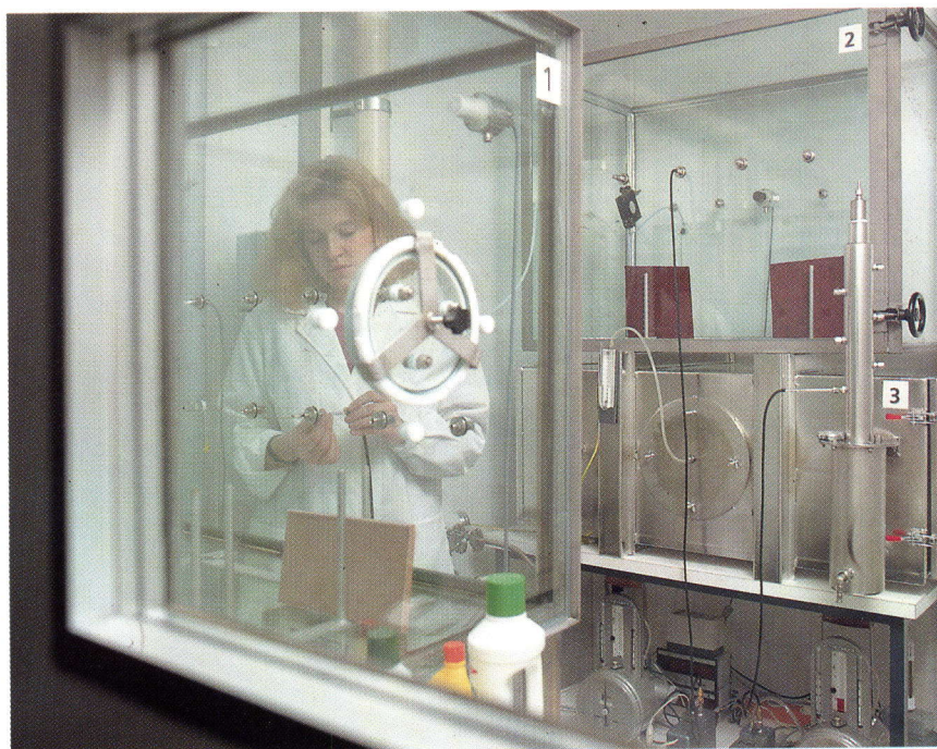
Thermostated room with three chambers, two made of glass and one of stainless steel, for the measurement of organic emissions from building materials, household and hobby products
