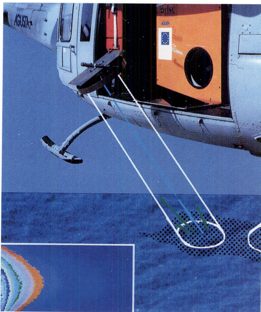
Single shot spectro-temporal measurement performed from the helicopter operating at 300 feet. The two bright spectral lines are the backscattering signal (355 nm) and water Raman diffusion signal (404 nm); the spectrally broad signal is the fluorescence of the dissolved organic matter.
