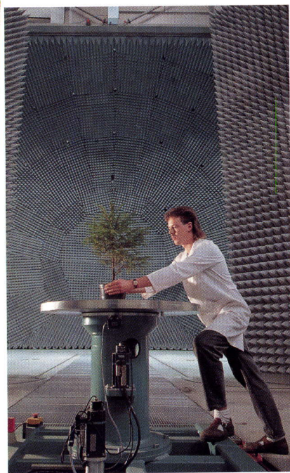
Looking from the outside into the Microwave Signature Laboratory; foreground the target positioner with a small tree and operator.
