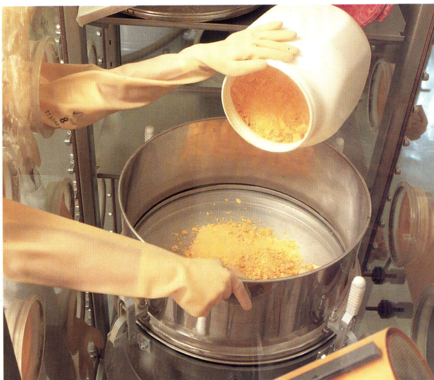
Sieving of organic material (e.g. orange juice powder) under controlled atmospheric conditions
