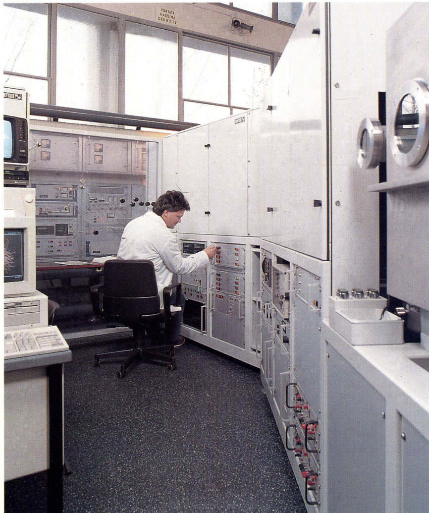
Surface Modification Centre: The high current ion implanter
