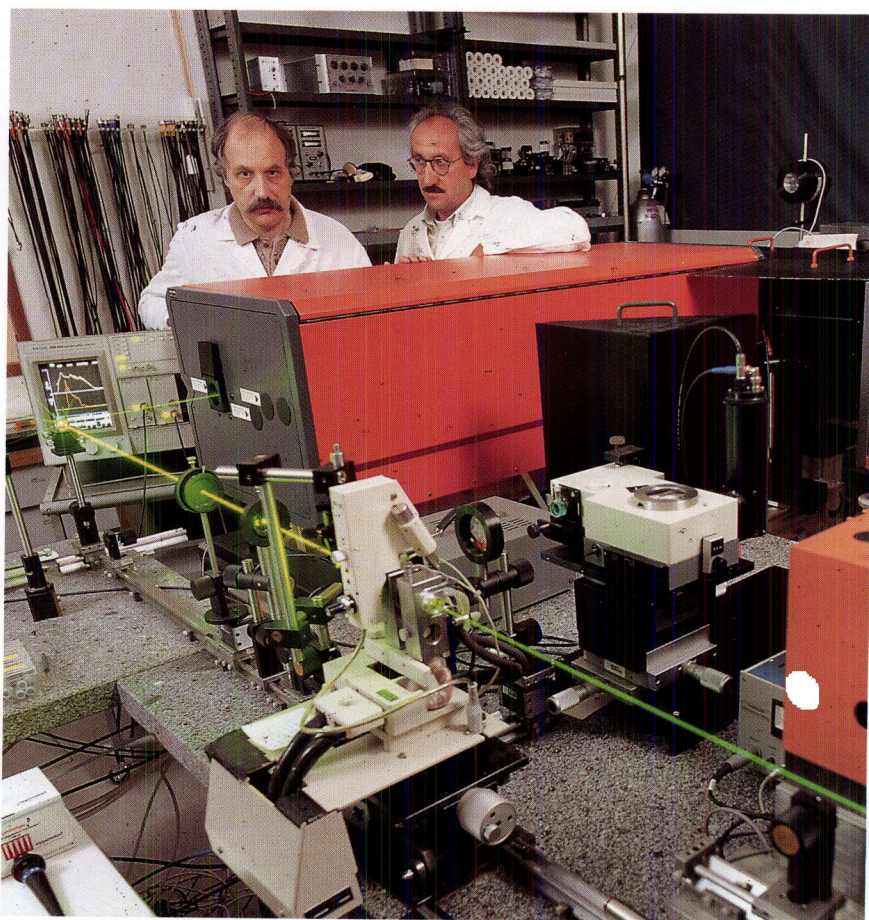
Three lasers are shown which are used to excite fluorescent light from atoms in a commercialized graphite furnace (in the centre).
