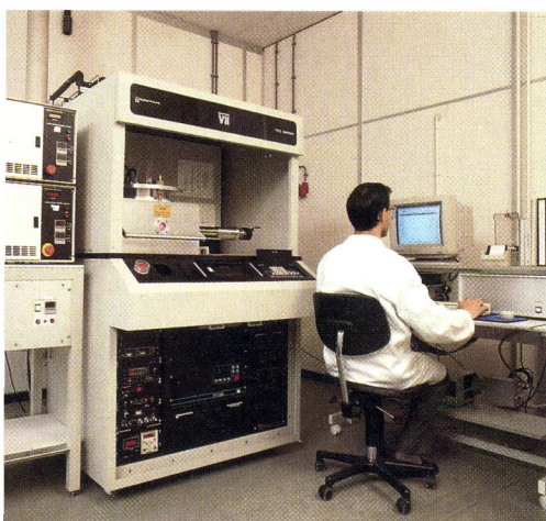
Radio frequency plasma assisted chemical vapour deposition reactor with data acquisition system and in situ plasma diagnostics of the Advanced Coatings Centre
