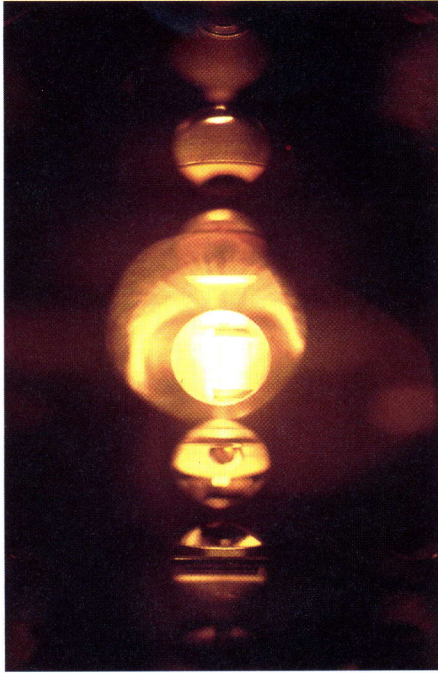
Ionizing silicon for high precision-high accuracy analysis of silicon traces
