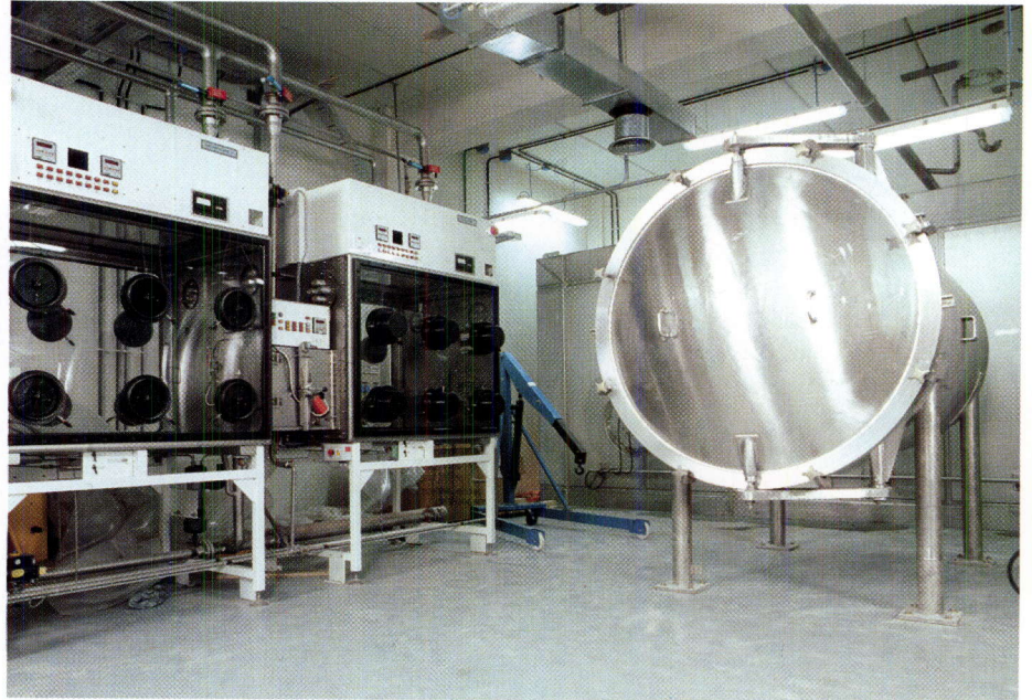
View of ETHEL's 5 m 3 Small Caisson tritium containment ("climate chamber") and associated glove-box suite, with 350 m 3 Large Caisson in the background
