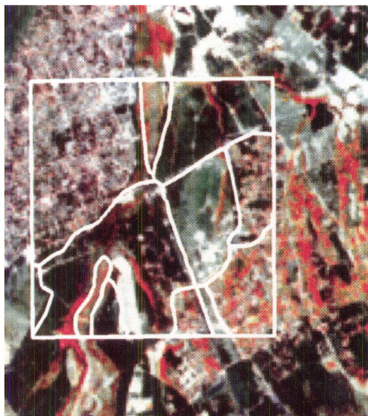
Land cover change; overlay of the CORINE land cover map with the colour composite Landsat Thematic Mapper image for a test site in Portugal
