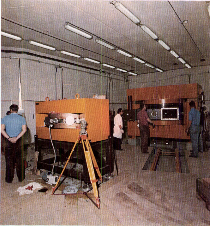
Figure 9 left: Thermonuclear fusion technology programme: View of the cyclotron hall during the assembly of the accelerator and the switching magnet.
