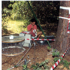
Parts of the JRC cuvette system to measure biogenic emissions of trace gases from oak/pine branches during the BEMA Campaign (June 93 Rome).
