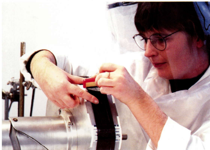
Fabrication of preforms for fibre-reinforced ceramic-matrix composites
