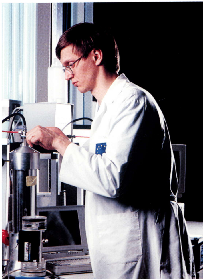
Set of laminar photochemical fluor reactors for the study of aerosol formation from the gas phase
