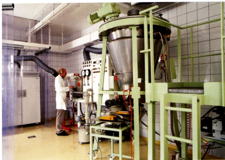
Installation for grinding, mixing and sampling to be used for the preparation of high quality reference materials
