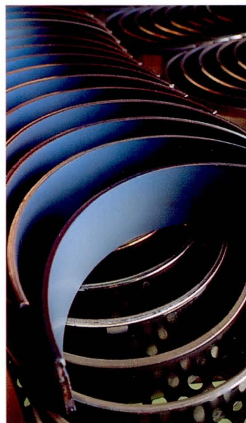
High-performance Cu-Pb sliding bearings: making large diesel engines more efficient.
