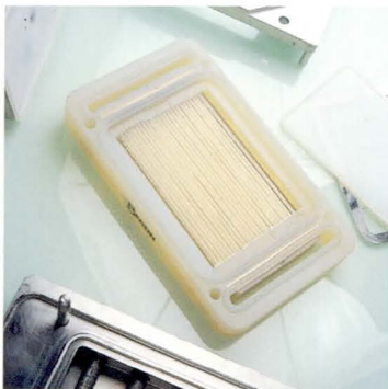
The flat configuration of the new bioreactor allows it to be scaled up in size by a factor of 100.
