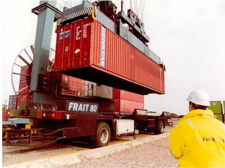
FRAIT: bringing high-speed automated container handling to ports without expensive guide path systems. Photo: Kevin Phillips
