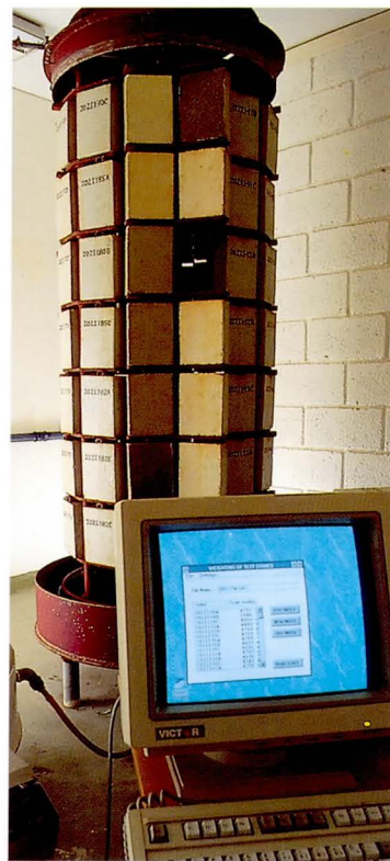
The 'Spray-Dry' towers simulate different weather conditions in the laboratory to test a wide range of concrete coatings.
