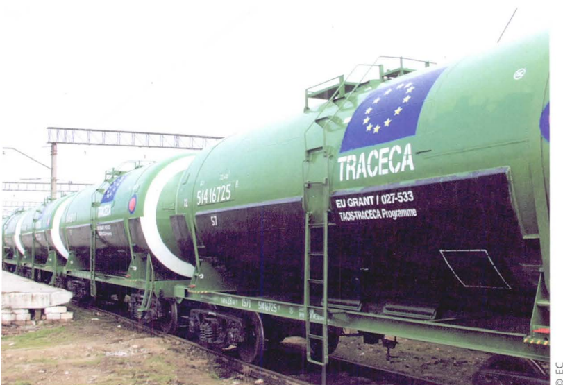
Arrival at Azerbaijan State Railways of 102 oil tank wagons purchased with an EU grant under the Tacis-Traceca programme. Each tank wagon will transport a 65 tonne liquid consignment and is equipped with a modern heating system
