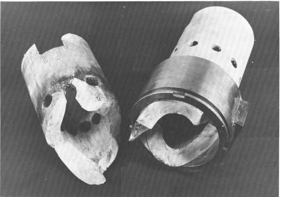
Figure 3.5 Remains of the ceramic diesel engine
