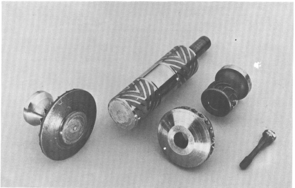
Figure 2.14.2 Turbomachine rotor after fracture of brazed joint at high speed
