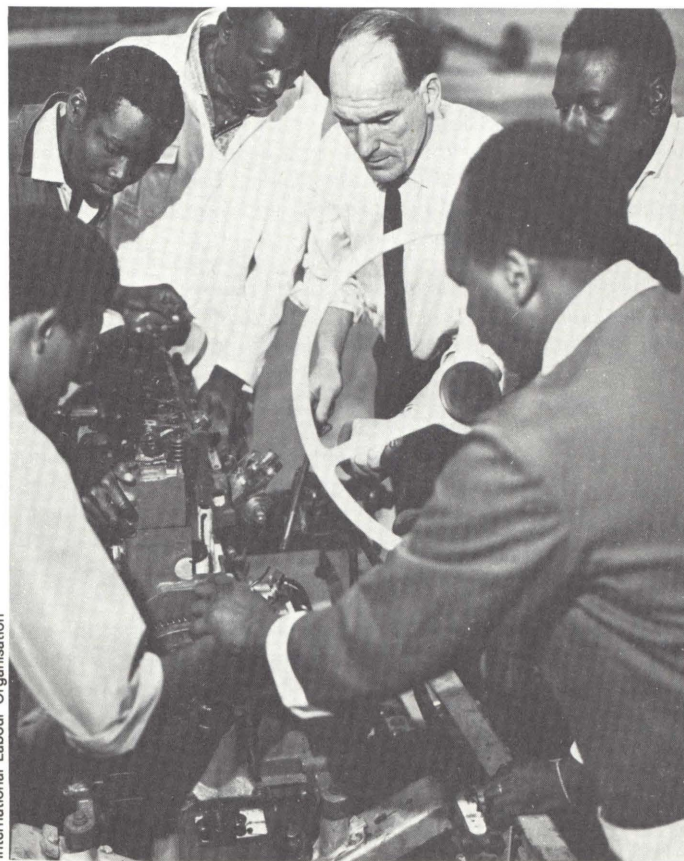
Trainees examine a cross section of an engine in Nairobi, Kenya.
