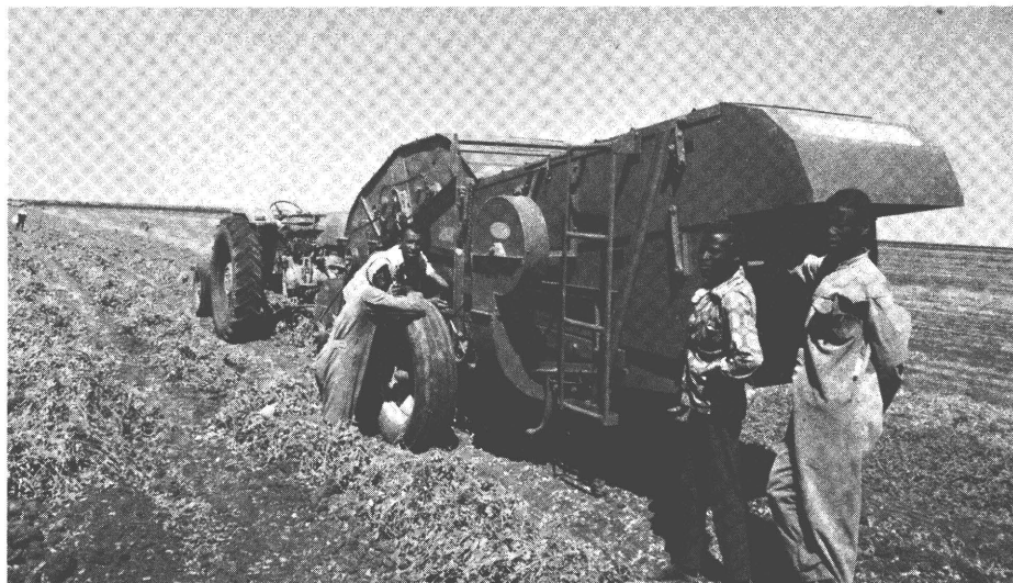
This modern harvester lifts the bushes, strips the nuts from the haulms and bags them
