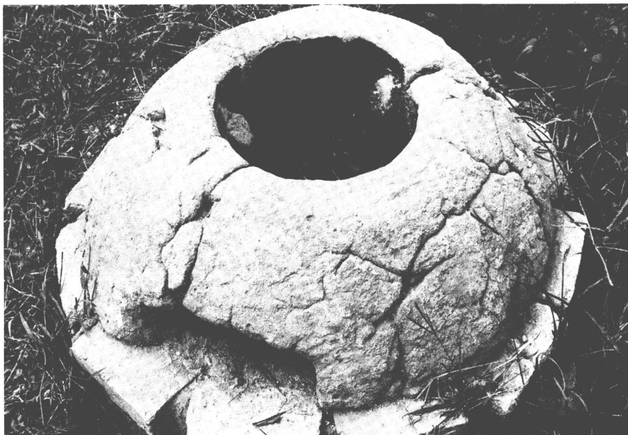
A simply-made oven that can save more than half the fuel usually burnt
