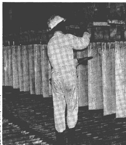
Final stage of the extraction of copper from tailings using electrolysis at the Nchanga mine, Zambia
