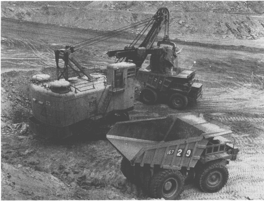
Two types of machines used in extracting and transporting copper ore. Each truck weighs between 85 to 120 tonnes and costs about one million US dollars
