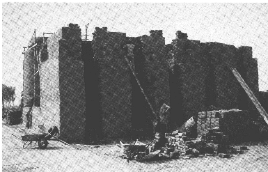
Brick kilns between the Senegal River and the hospital site. The sand and clay used to make the tiles come from the river
