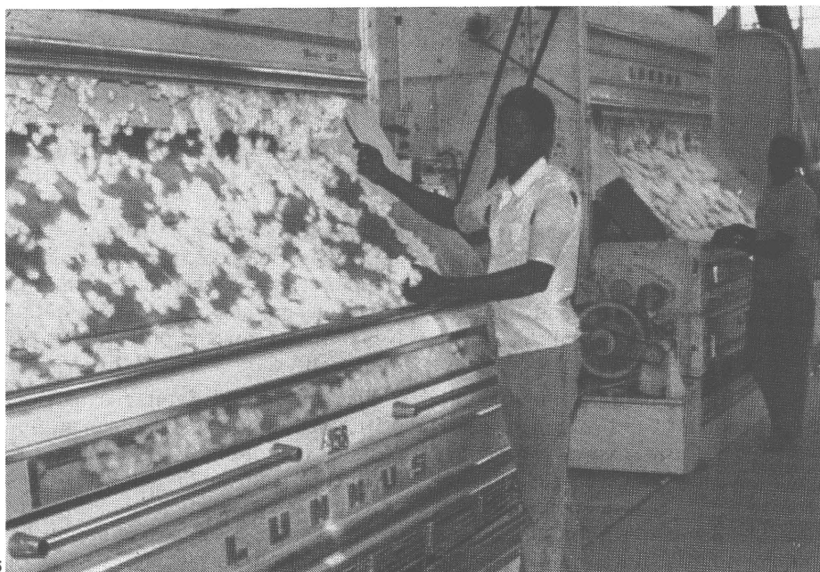
A ginning machine, the first stage of cottonseed processing
