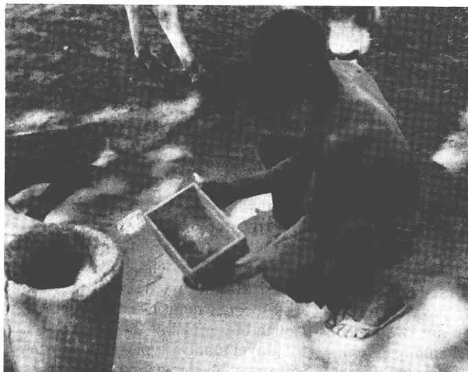
Sieving ground ore to obtain a fraction suitable for sluicing
