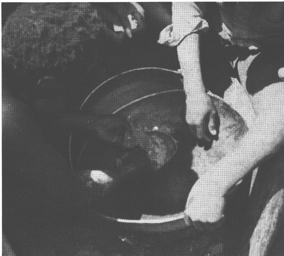
Amalgamating the gold concentrate with mercury by rubbing in a fine cloth
