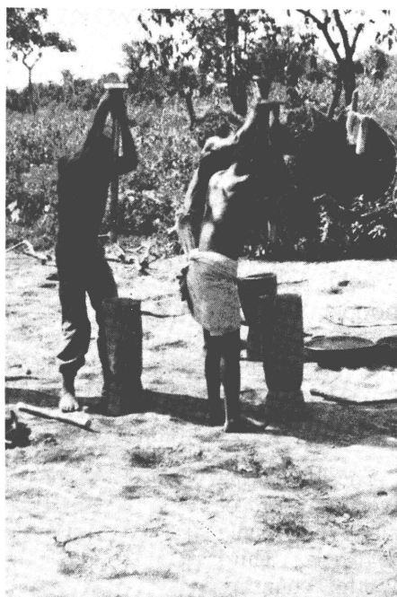
Crushing the broken ore in grain mortars, using axle shafts
