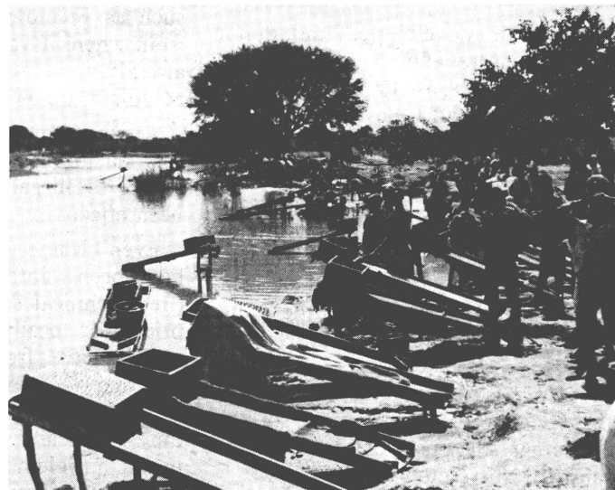
Sluicing, with sacking on the strakes as a collecting surface, to produce a gold concentrate on an African river
