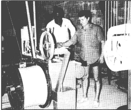
The French partner, Mr. André Vayrac (right) with a plastic coating extruder, for electric wire.
