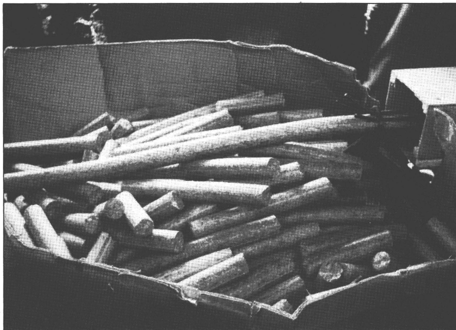
Combustible briquettes produced from coffee husks in a CDI-assisted project in Rwanda.
