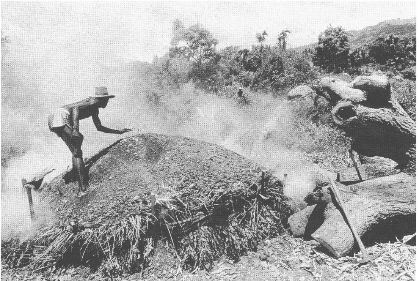
Traditional charcoal making in Haïti, in an earth kiln
