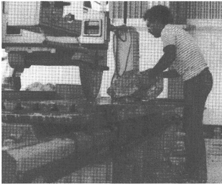
CDI-sponsored Italian marble expert, Mr. Faini, cuts the first boulder with the new slabbing machine in the Jamaican plant.
