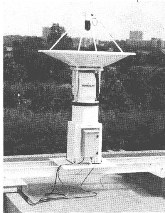
The NOAA/AVHRR satellite data reception station has just been installed at the AGRHYMET Centre
