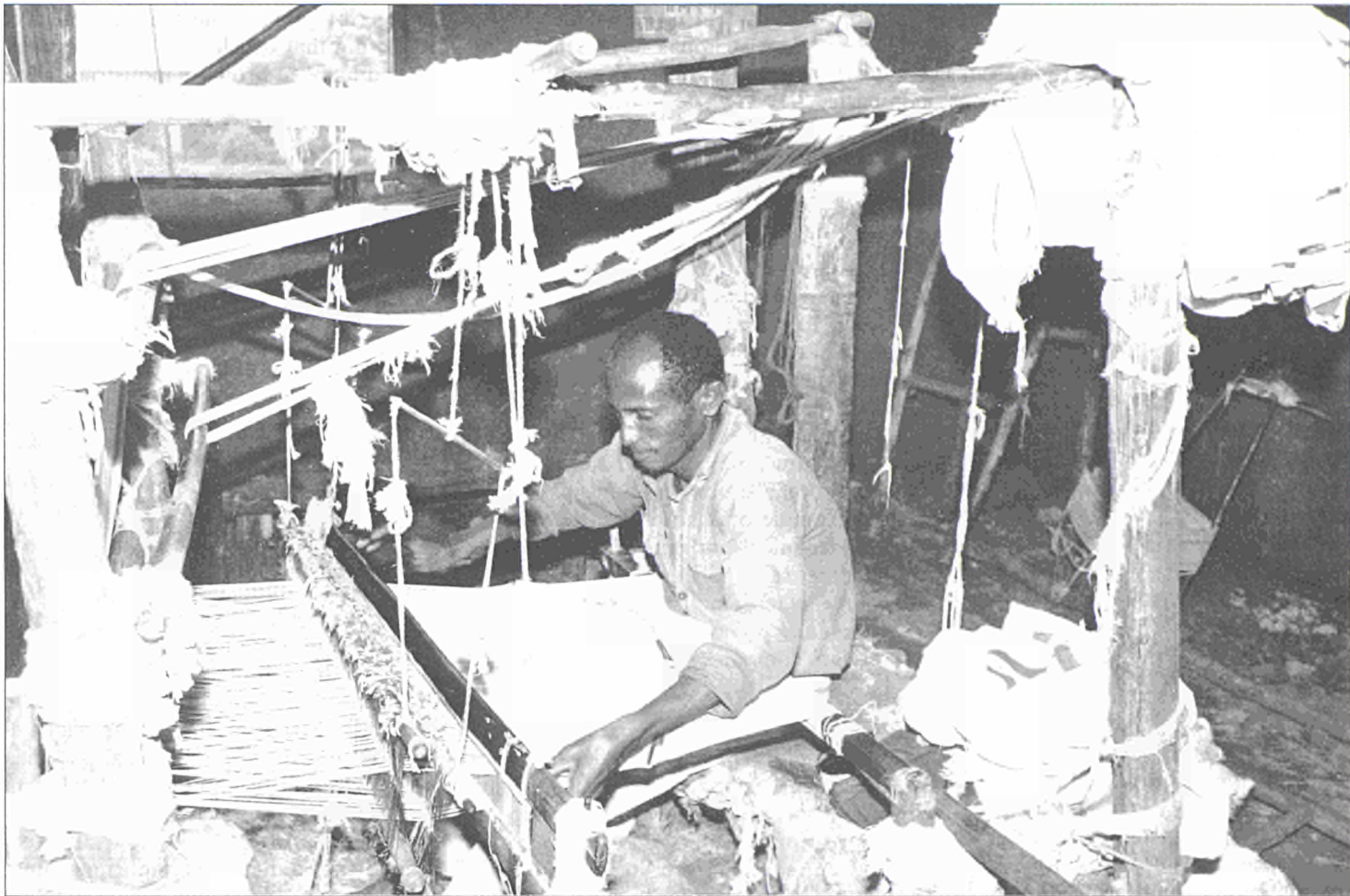
A rudimentary traditional loom in Addis Ababa. 'Technology is also to be found within people'
