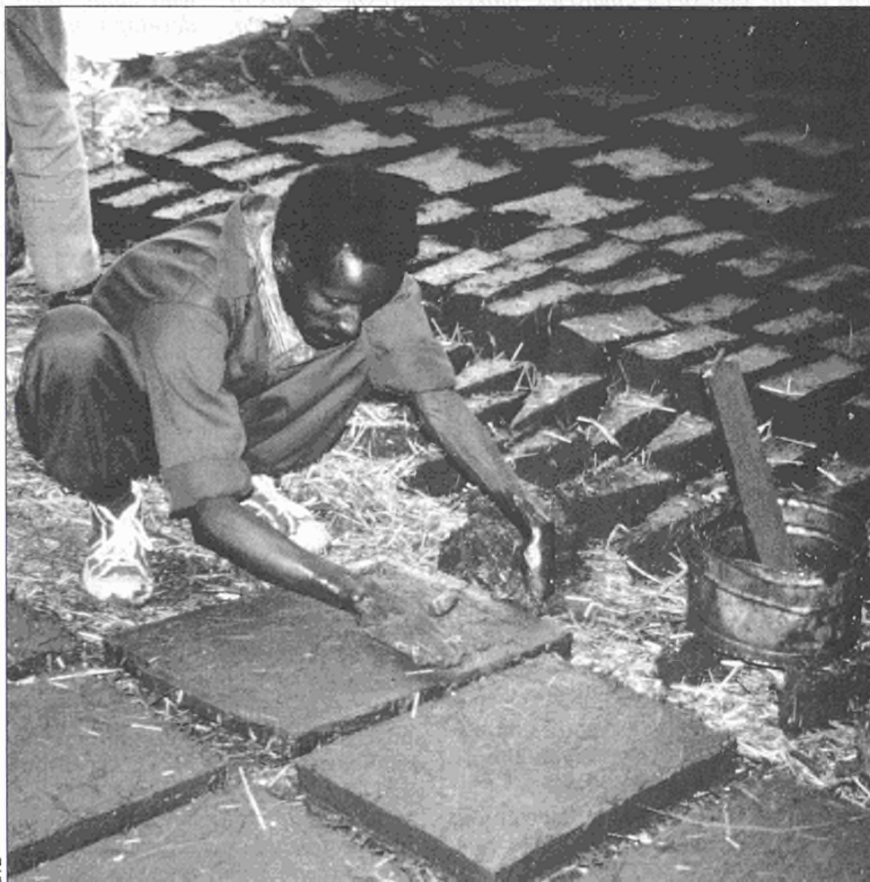
Making clay bricks is part of the start-up training in house building which GTZ gives ex-soldiers in Ethiopia
