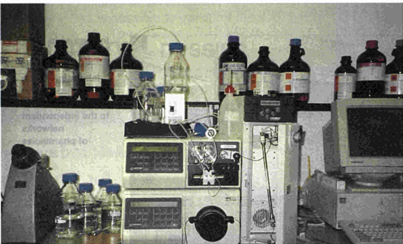
HPLC (substance quality control). This type of modern, high-performance equipment will eventually replace the antiquated machinery currently in use
