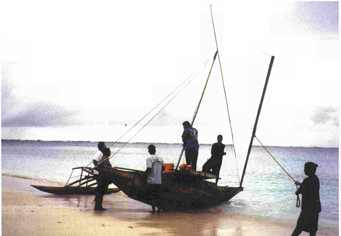
The traditional outrigger canoes of the Marshall Islands are noted for their asymmetrical hulls and a reversible mast that allows fast sailing close to the wind. Majuro Lagoon
