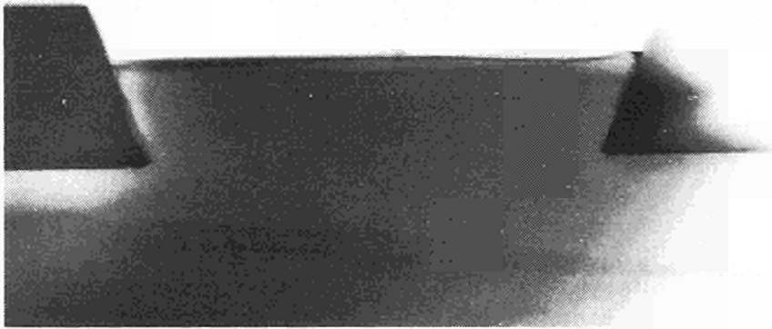
Fig. 10 : TEM cross-sectional view of SEG filling showing excellent crystallographic quality
