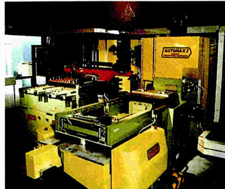
The CNMA demonstration cell at the 1987 Hannover Fair, incorporating a machining centre, automated tool management with a pick and place robot, and a manual job preparation area, all linked by an automated transportation system (ESPRIT Project 955).
