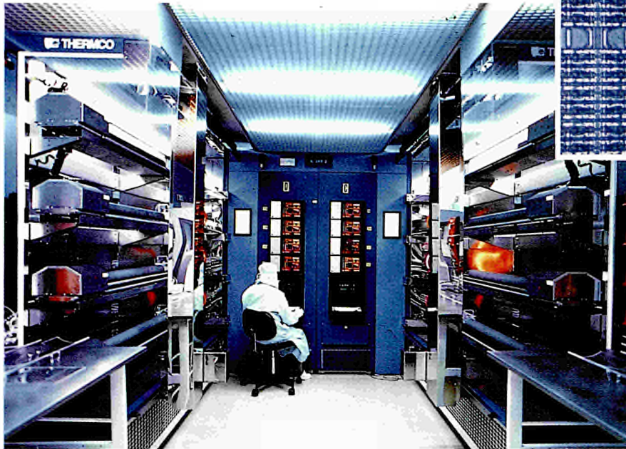
The new R&D facilities of SGS-Thomson Microelectronics has just been completed in Italy. This lab is equipped with a 2500m 2 class-1 clean room, where full automation of process islands is being implemented (ESPRIT Project 1551). On this line STM is developing a CMOS technology devoted to ASICs manufacturing (ESPRIT Project 554). The inset illustrates a few cells of memory, designed for fine tuning of the process
