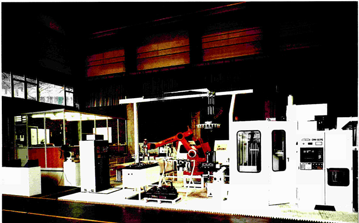
A fault tolerant flexible machining cell in Mondragon in Northern Spain using multi-sensor inputs, a modular universal monitoring computer, and model based diagnostic techniques (ESPRIT Project 504).
