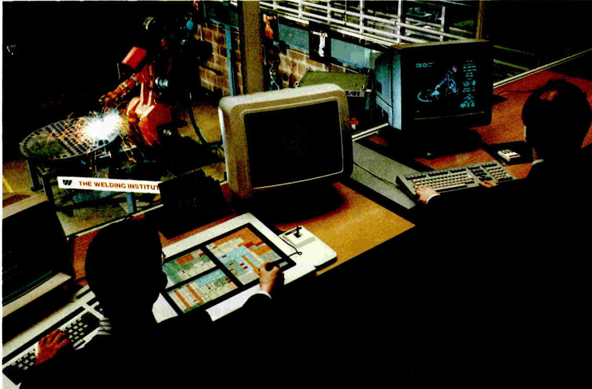
Welding in progress in the FMS weld cell constructed at TWI, Cambridge. The centre CAD screen shows 3-D product data, which is transferred to the off-line programming facility shown on the right (ESPRIT Project 595, The Application of CIM to Welded Fabrication, involving the Welding Institute, Aalborg Shipyard Ltd, Italsiel SpA, Università di Genova, Odense Steel Shipyard and the Danish Welding Institute). (Acknowledgement: The Welding Institute).
