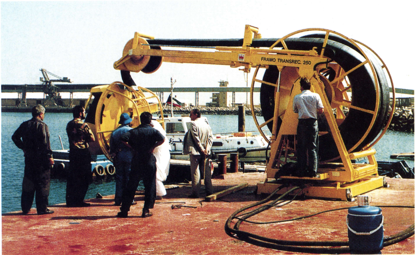
Fig 2 A Framo Transrec 250 system with a treatment capacity of 250 tons/hour
