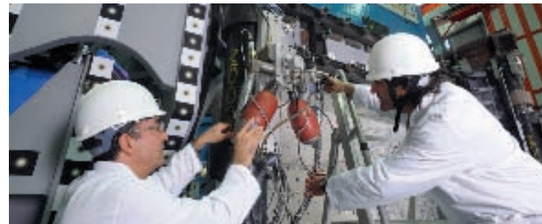
▲ Setup of a large-scale structural test (industrial building shear-wall) at the European Laboratory for Structural Assessment (ELSA) Laboratory: Hydraulic high-pressure hose connection to the actuator's servo-valve.
