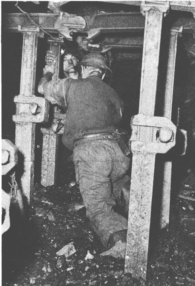
Methods of roof support in coal mines is one of the projects being undertaken through the Community's technical research program. Here metal props are being shifted in the LaHouve mine in the Lorraine coal basin, France.
