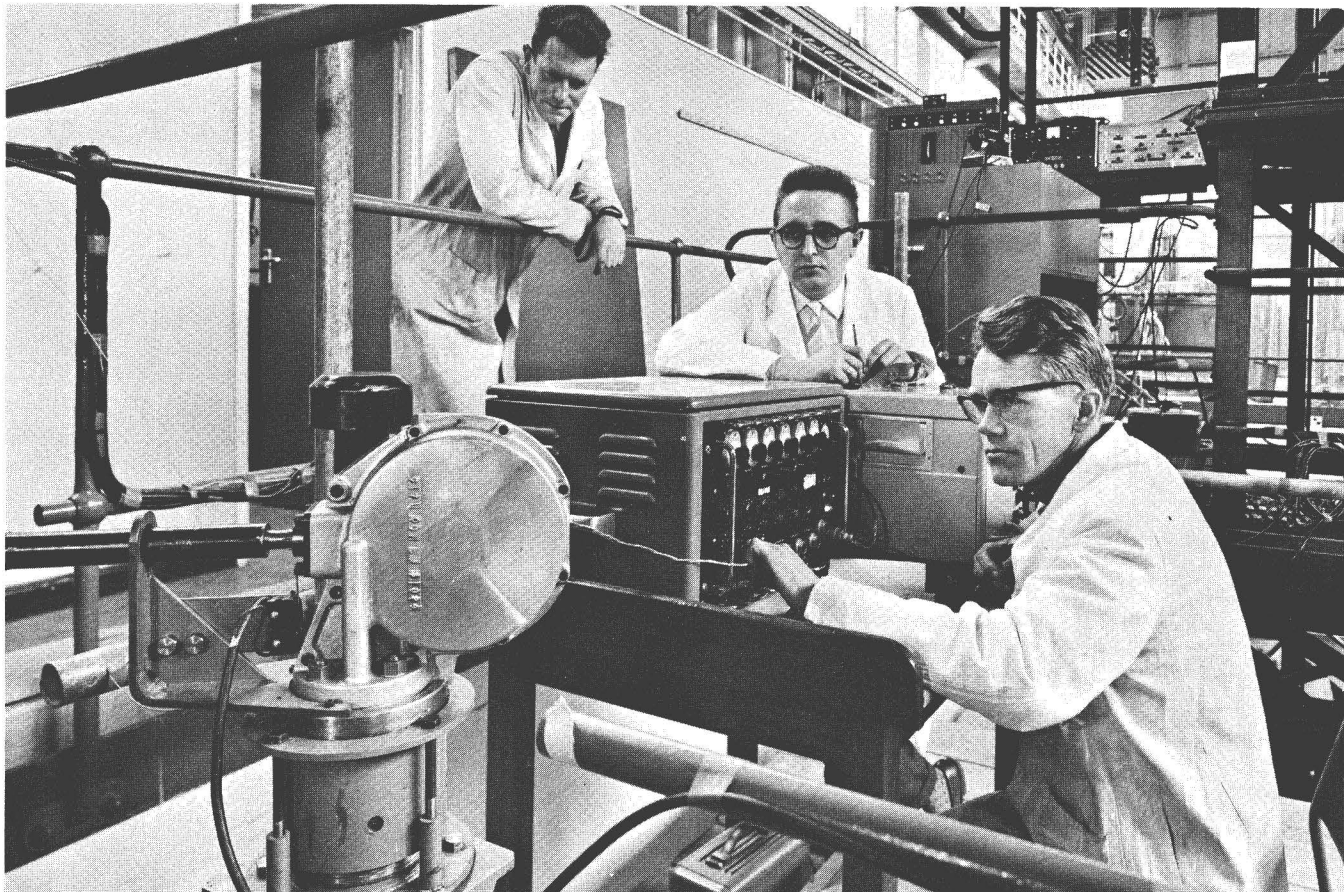
Dragon Project scientists from Britain, France and Norway are here testing a control-rod drive mechanism. The international staff working on this program is drawn from 12 different countries.
