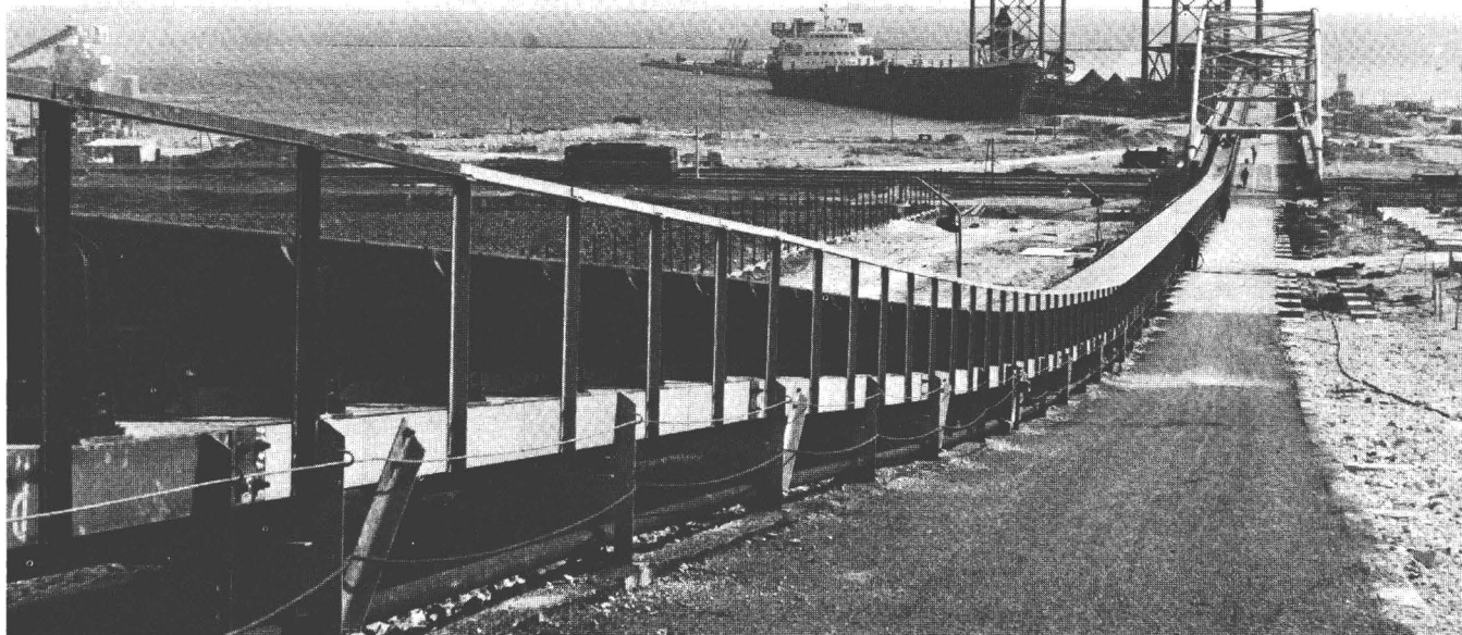
Link to the Sea: A conveyor belt connects the Taranto steelworks to the industrial harbor. Construction of the steelworks was aided by funds from the ECSC High Authority and the European Investment Bank to lift the economy of the under-developed Taranto-Bari area of southern Italy.
