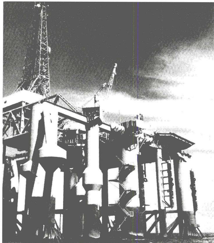
Floating, semi-submersible drilling rigs are being used to tap offshore natural gas deposits.
