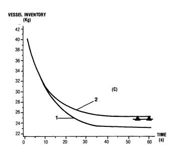
Fig. 11 - Comparison between SAFIRE calculations and measured data concerning the water blowdown test "2" performed with the MPMC-TF
