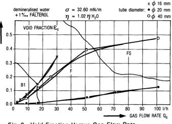
Fig. 3 - Void Fraction Versus Gas Flow Rate
