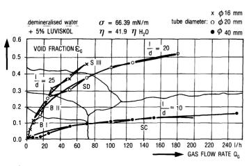
Fig. 4 - Void Fraction Versus Gas Flow Rate
