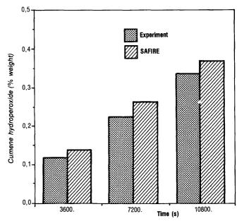
Fig. 15 - Comparison between SAFIRE calculations and experimental data concerning a chemical reaction (cumene hydroperoxidation)
