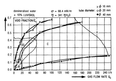
Fig. 5 - Void Fraction Versus Gas Flow Rate
