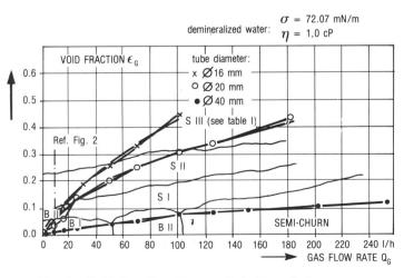
Fig. 1 - Void Fraction Versus Gas Flow Rate
