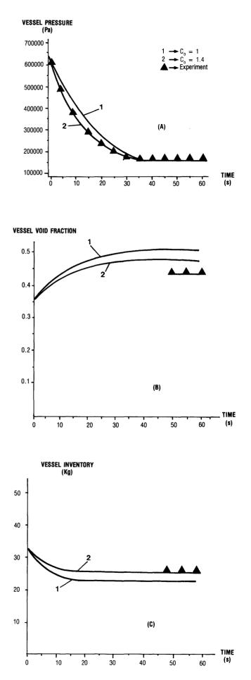
Fig. 10 - Comparison between SAFIRE calculations and measured data concerning the water blowdown test "1" performed with the MPMC-TF
