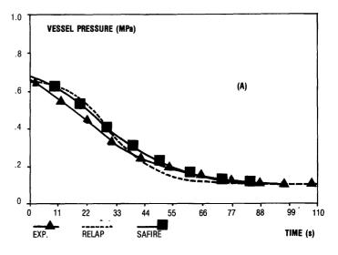
Fig. 12 - Comparison between SAFIRE, RELAP5 and experimental data concerning the water blowdown test "3" performed with the MPMC-TF
