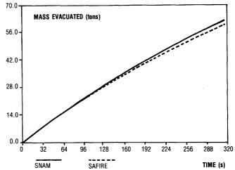
Fig. 14 - Acid storage VESSEL voiding - mass evacuated versus time
