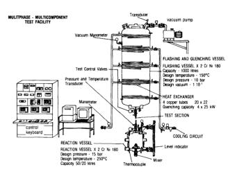
Fig. 6 - Multiphase - Multicomponent Test Facility
