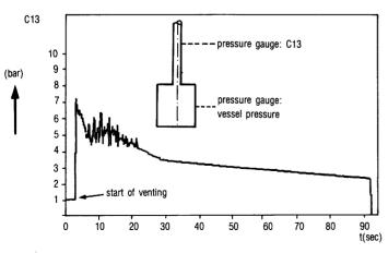
Fig. 8 - Depressurisation history (pressure in the test section, pressure gauge C13)
