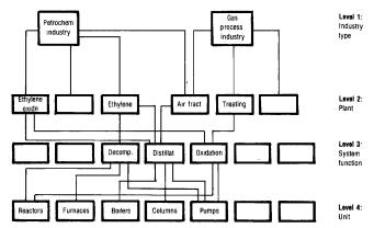
Fig. 12 - Basic criteria for plant classification
