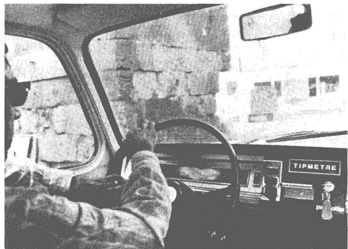
Each TIP subscriber receives an ignition key that fits every car. Plastic tokens are then fed into the meter on the dashboard.
