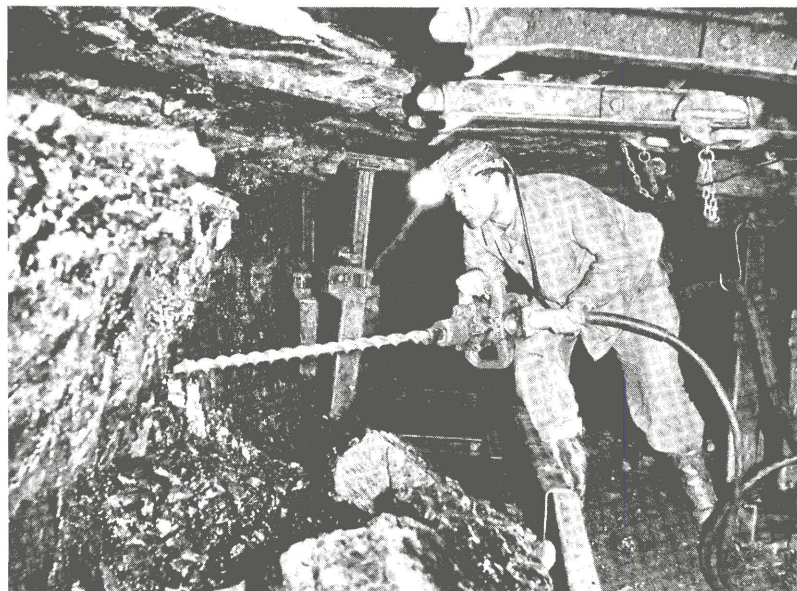
The EC's coal industry cannot compete on a worldwide basis, but many mines are kept open for national security and social reasons. At La Houve, a mine in the Lorraine basin, a coal miner drills holes with an electric rotative perforator.
