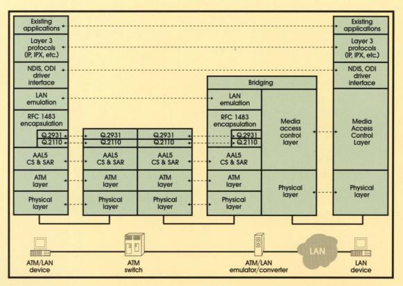
Figure 3 Layered Structure of a LANE over ATM
