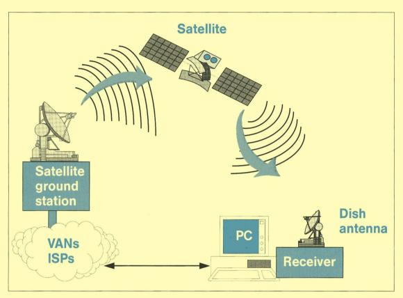
Figure 5 Example of High-speed Communication via Satellite and PC with Dish Antenna
