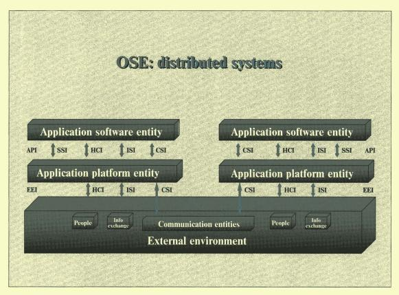
Figure 13 OSE Logic for Distributed Systems
