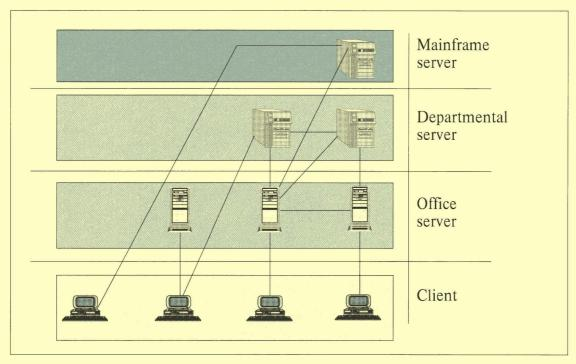
Figure 7 An Example of 4-tier Client/Server Architecture
