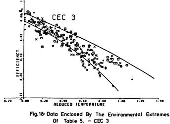
THE SCATTER OF DATA WAS ATTRIBUABLE TO SYSTEMATIC ERRORS IN MEASUREMENT AND METHOD OF TESTING. SCATTER MAY ALSO HAVE BEEN INTRODUCED BY VARIATIONS IN THE PROPERTIES OF THE DISTRIBUTED COLLECTORS. THE RESULTS OF TESTING USING SIMULATED SOLAR RADI-ATION WERE MORE REPRODUCIBLE THAN THOSE FOR OUTDOOR TESTING.
