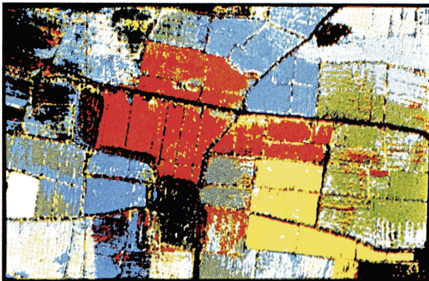
Fig. 24 - Classification results of rice varieties with ML method after data compression from 8 to 5 dimensions, by principal components analysis.
