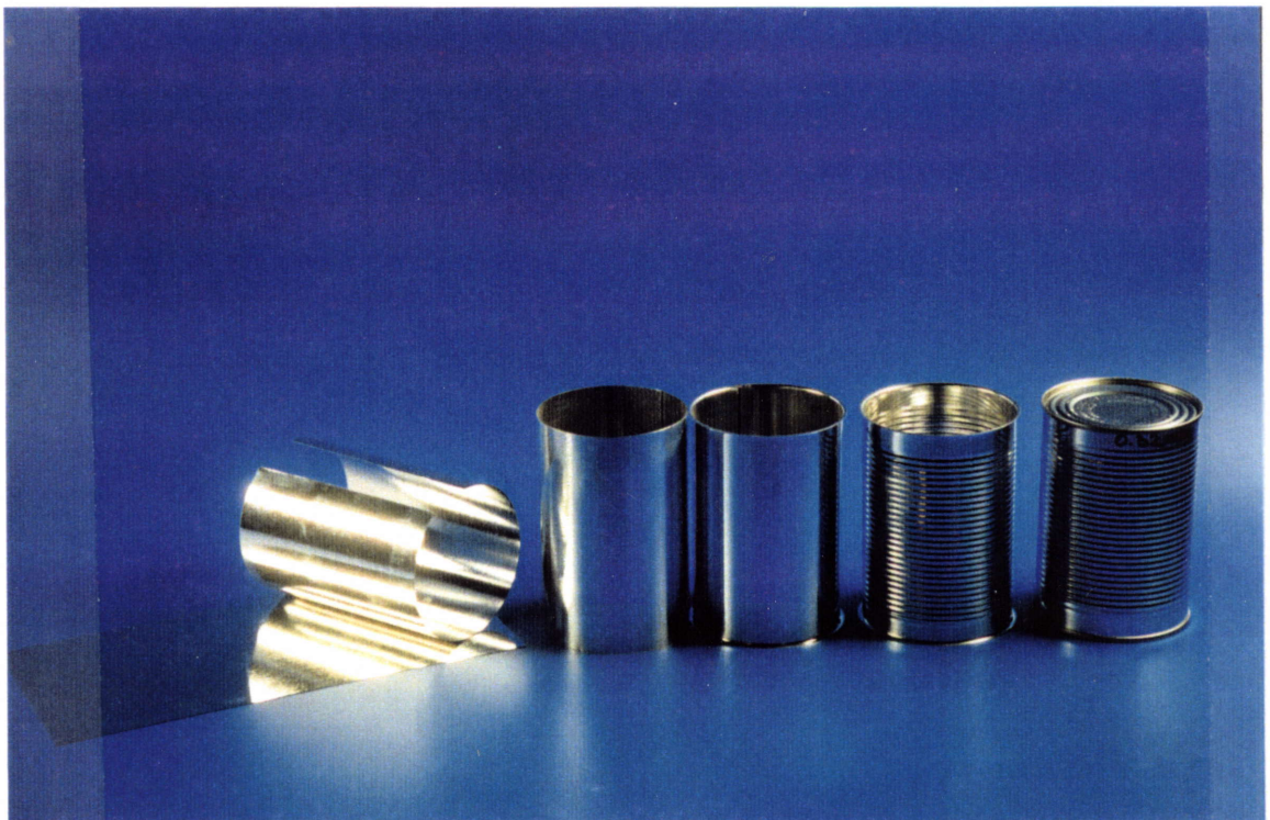
Photo 1 : Production steps for the welded can
