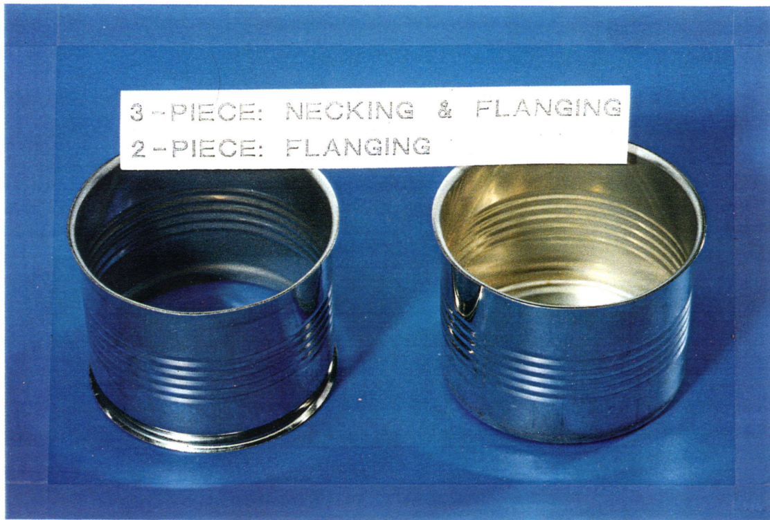
Photo 10 : Products after necking and flanging of 3-piece can and flanging of the 2-piece can
