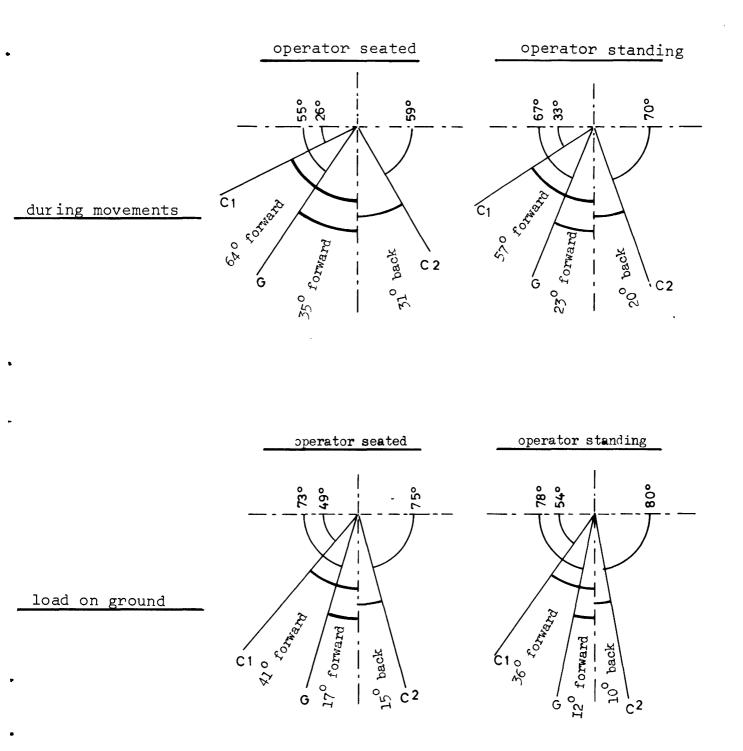
diagram summarizing angles of vision in two working situations and with operator seated or standing
