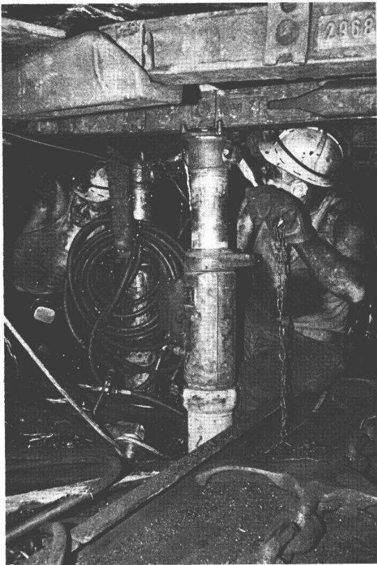
Fig. 38 - Putting intermediate pick into position
