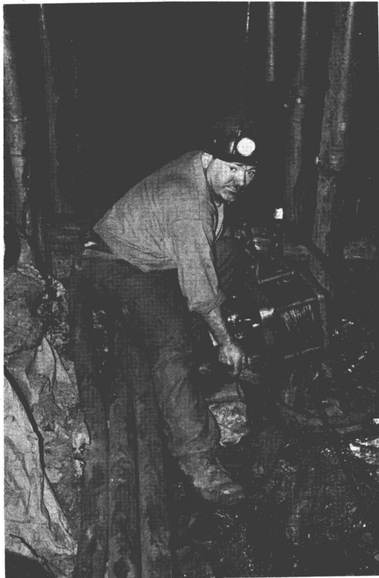
Fig. 36 - Winch for drawing props and caps
