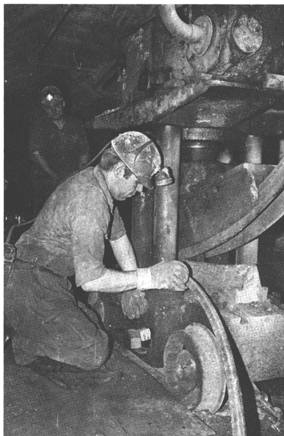
Fig. 33 - Bending press for straightening support sections
