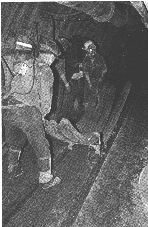
Fig. 32 - Bent support sections delivered from timber-withdrawing workings are unloaded by hand
