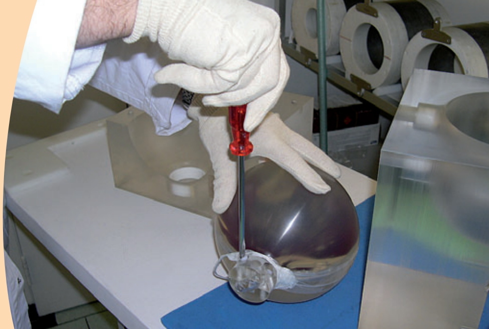
Figure 16 - Gel dosimeter being fixed into liver holder prior to irradiation
