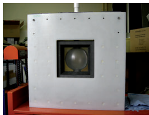
Figure 15c - Beam-eye view of final configuration, covered with polyethylene sheet
