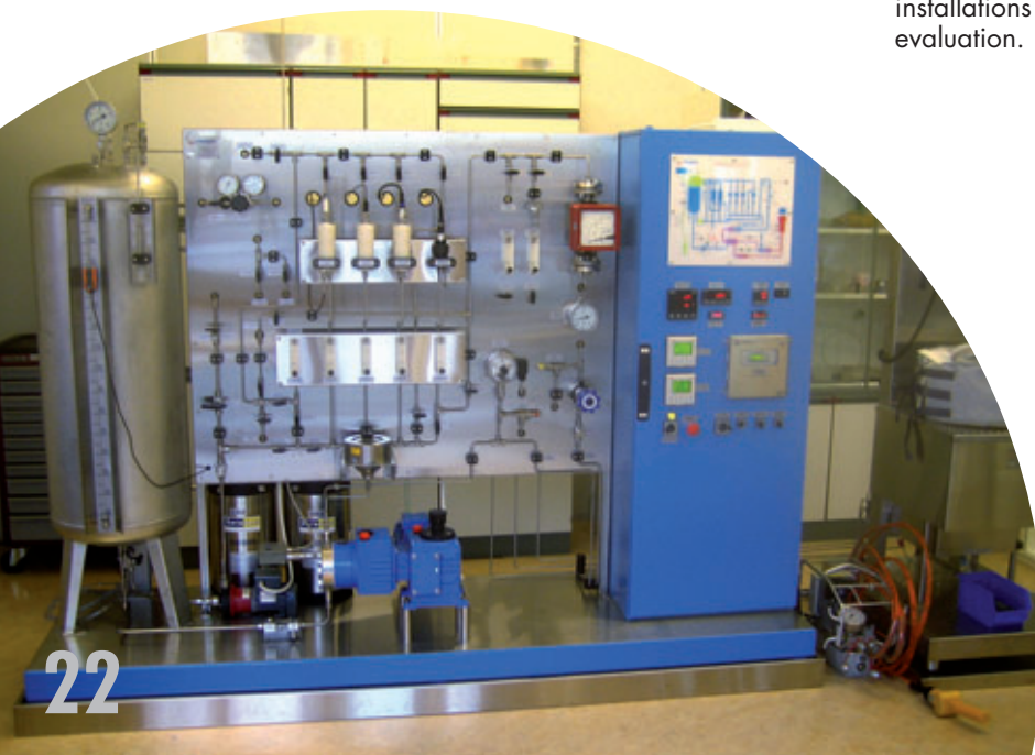
Figure 19 - Supercritical water recirculation facility for material tests
