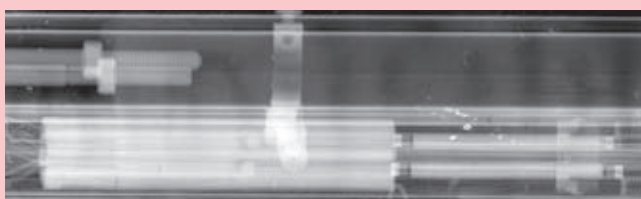
Figure 22 - Neutron radiography of the TRIO rig taken during cycle 2005-08 on 7 th September 2005 (upper section)
