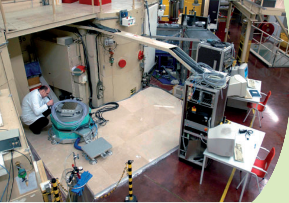
Figure 37 - HFR/HB5: new diffractometer for residual stress analysis installed on "Tanzboden" floor
