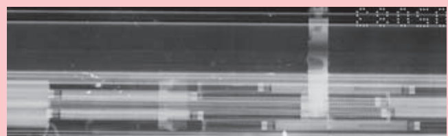
Figure 23 - Neutron radiography of the TRIO rig taken during cycle 2005-08 on 7 th September 2005 (middle section)
