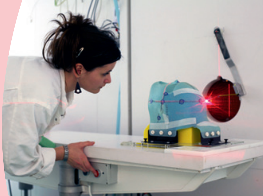
Figure 25 - Positioning check using the laser beam and patient mask prior to dosimetry measurements
