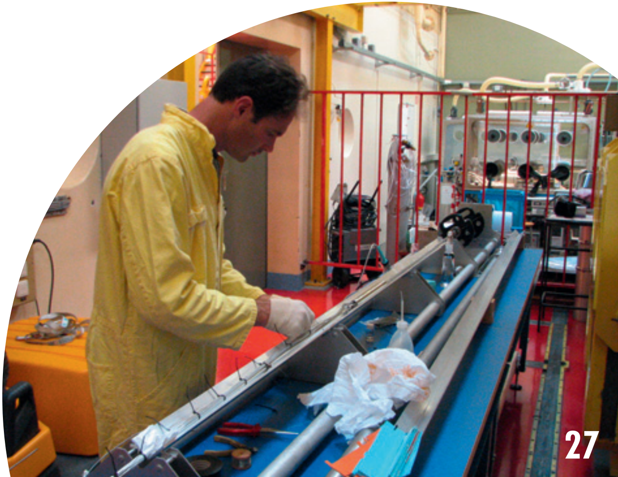
Figure 34 - Assembly of the experiment for graphite irradiation
