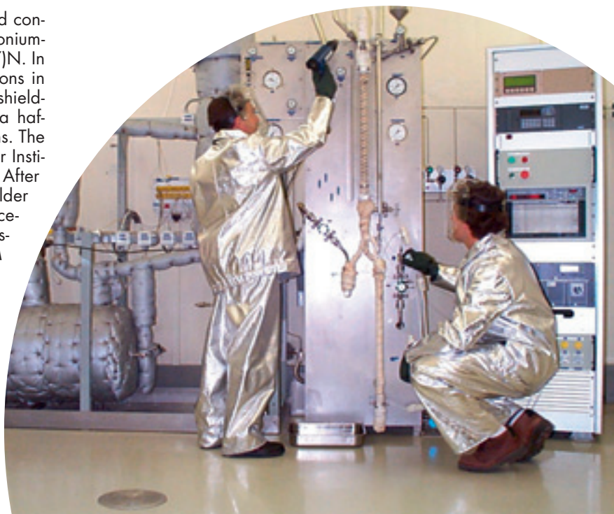
Figure 43 - Sodium filling of the CONFIRM irradiation
