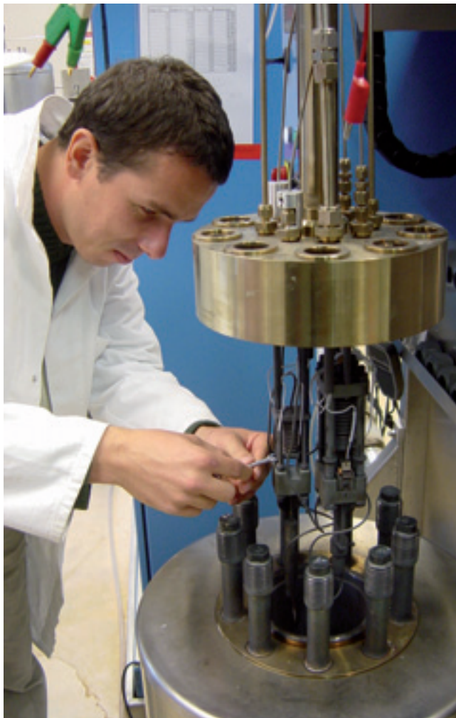
Figure 14 - AMALIA Autoclave for Stress Corrosion Cracking (SCC)
